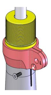
13. Install the spring perch and black plastic isolator disc (in Coil-Over Hardware Kit) as shown. Adjust the perch to about 3/8" up from bottom. This will be the starting ride height setting, and should get you close to Dinan's target ride height. Snug the 6mm screw to lock the perch into place.
