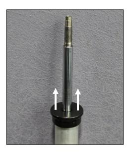
21. Locate the D112-0078 Dinan Shock Cap and D671-0254 O-ring in the hardware kit. Insert the O-ring into the groove inside the cap, and install cap onto shock. If needed, add a small amount of lubricant to ease assembly.
