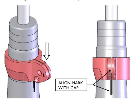
Locate the two Front Threaded Perch Assemblies. These are the same for left & right. Verify that the O-rings are properly located in the grooves as shown in figure.
