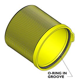
10. See figure below. Slide the threaded sleeves onto the struts as shown. Turn the sleeve to align the tab with the notch in the endlink mount. Note that the O-ring may make the sleeves spring upward slightly. This is OK.
