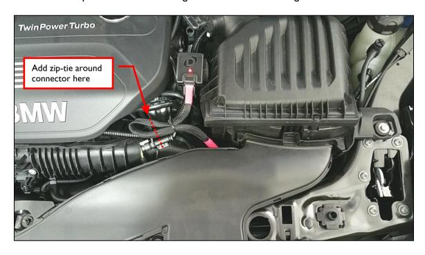
10. Reinstall the air intake duct.
