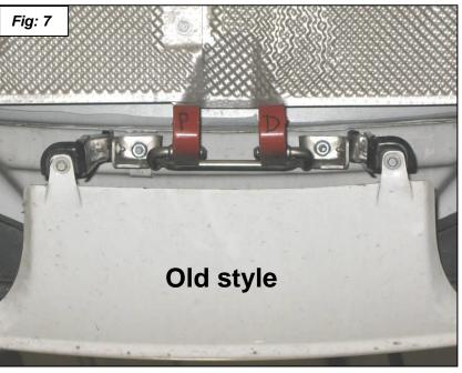
12. Remove the front rubber hangers with mount from the stock mufflers by pulling them off the wire hangers on the muffler. Insert the 10mm x 65mm bolt as shown. Clamp in a vise and run a 10mm copper locknut down to
