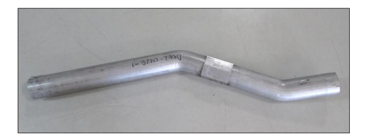
1. Support the exhaust securely with a jack or a stand, then cut the stock mid-pipe at the front end of the resonator as shown in **Figures I & 2**. Before cutting the stock mid-pipe, hold DINAN mid-pipe underneath stock mid-pipe to verify the stock pipe will not be cut too short!
