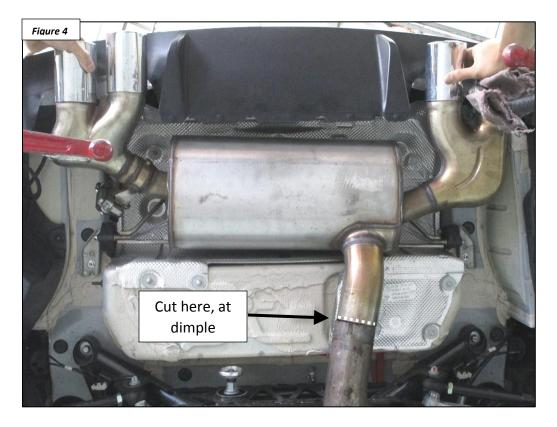
3. Install the DINAN mid-pipe with clamps as shown below.
