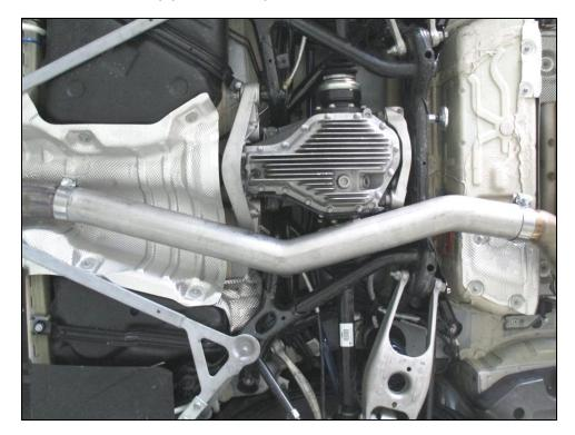
4. Using **Figure 5** be sure to check that there is enough slip fit engagement. There should be no gaps exposed in the clamping slots.
