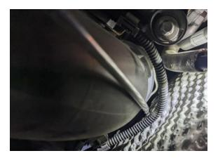
21. Raise clean air pipe, release connector (1) on heating element and disconnect.
