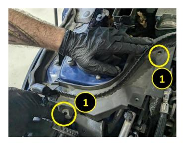
30. Position partition wall (3). Tighten screw (2). Attach expanding rivet (1).
