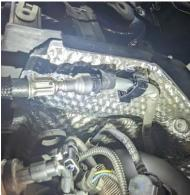
28. Install wire harness plate on the bulkhead.
