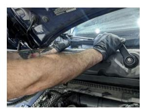
8. Loosen 1 Cap nut (1). Open 3 Locks (2) by turning them counter-clockwise.
