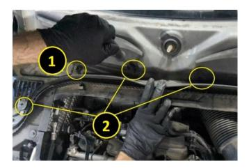
9. Unclip and remove the cover upwards from the holding rail.
