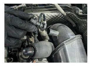
20. Unlock clamp at the turbo inlet.
