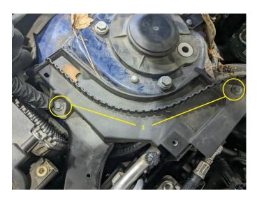
14. Unscrew the 3 screws and unclip fuel line from holder.
