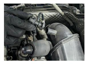
20. Unlock clamp at the turbo inlet.
