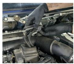
11. Release expansion rivet and release screw.
