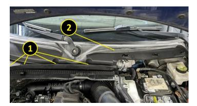
32. Join wiper arm and tighten with nut (2) to 26 ft-lbs. Install protective cap (1).
