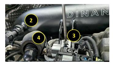
26. First connect the flex pipe (1) to air box and then to Dinan pipe. Ensure flex section orientation is as shown below. Tighten clamps (2) to 2.2 ft-lbs.
