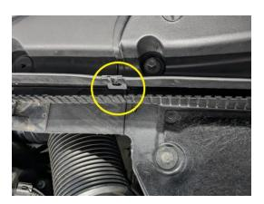
34. Install top bulkhead cover. Reinstall seal.
