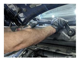
8. Loosen 1 Cap nut (1). Open 3 Locks (2) by turning them counter-clockwise.
