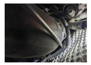
21. Raise clean air pipe, release connector (1) on heating element and disconnect.
