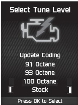
**STEP 5** - Selecting "Yes" will write the stock files to the vehicle and relock the DME. Select this option if you wish to completely remove Dinan software and return the car to factory configuration.
