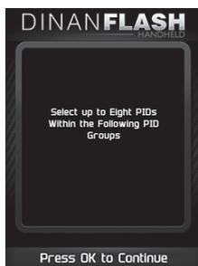
**STEP 5 - Select a PID Group, then select between 1 and 8 PIDs. Use the ◀ / ▶ arrows to switch between screens. OK to select.**
