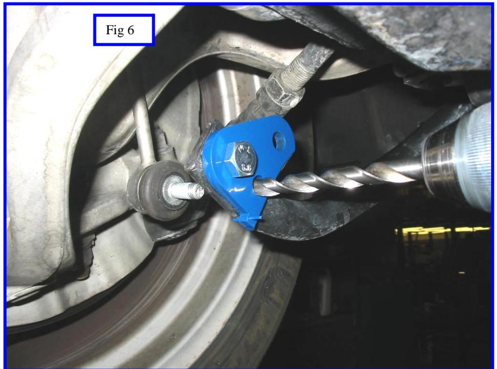
**one step with the 10mm bit, you will burn up the bit.** Make sure the plate does not move during drilling. (See Figure 6)
