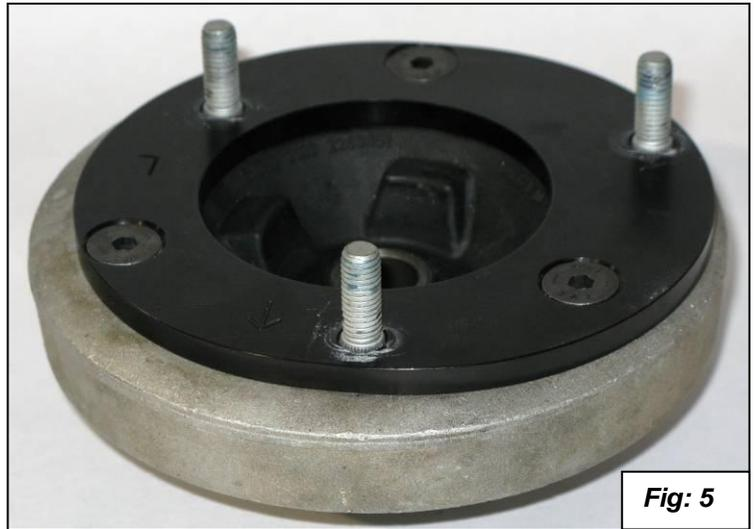
10. Carefully install the bearing assembly back onto the guide support and reassemble the strut assembly.
