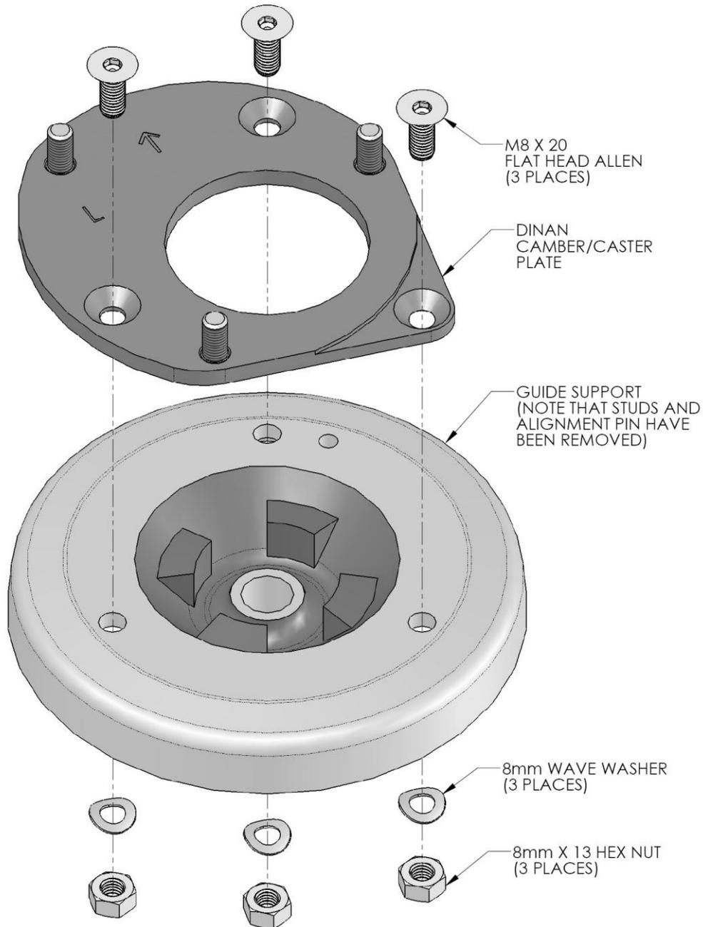
6. Install the assembled bearing plates onto the struts using the original hardware. Take care to install the Left plate onto the driver-side strut, and the Right plate onto the passenger-side strut.
