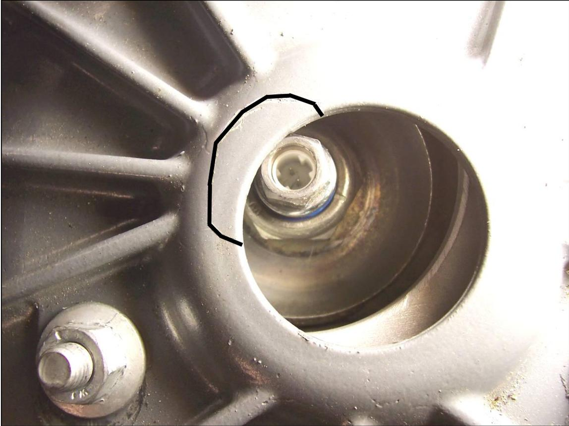
9. Unbolt strut from vehicle and cover any components below the strut tower to protect from debris. Using a die grinder or other suitable tool, enlarge the opening up to your scribe line.
