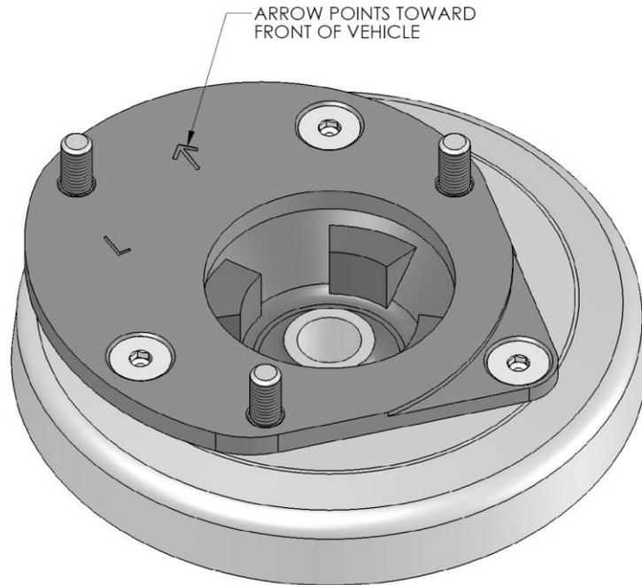
8. Clearance must be made in the strut tower for the electrical plug. Scribe a line that provides 1/16" to 1/8" of clearance around the plug (see figure below), when the strut is at the maximum negative camber position (see step 7).
