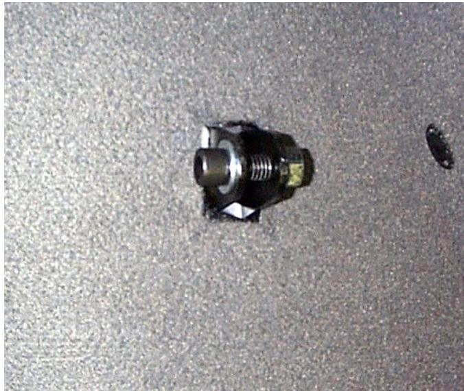
23. Install the center section onto the Allen head bolts and tighten securely. To maintain the finish on the endplates, hold flanged nuts with wrench while tightening the Allen-head bolts.
