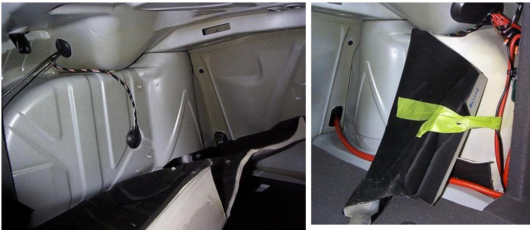
11. The Dinan brace will mount between the shock towers, just above the upside down "V" stamped into the towers.
