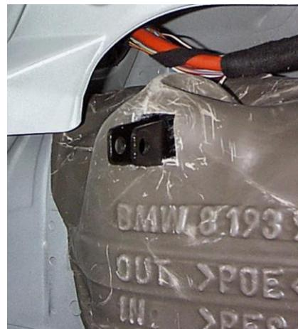
15. Slit and trim the carpet as required to go around the ears and install in reverse order from removal.
