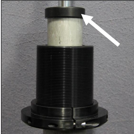
9. **NOTE:** Adjust the spring perch until it is approximately in the middle of the adjustment range. This location should set the vehicle at the approximate target ride height.
