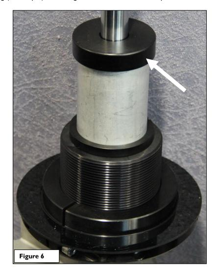
10. Locate the Front Shock Cap. It is engraved with a "L". Insert a D671-0158 Oring (see Step 4) into the groove inside, and install cap onto shock. See Figure 6.
