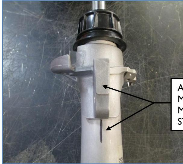
4. Once the tab locations have been marked, remove the plastic caps from the top of the struts. These will not be reused.
