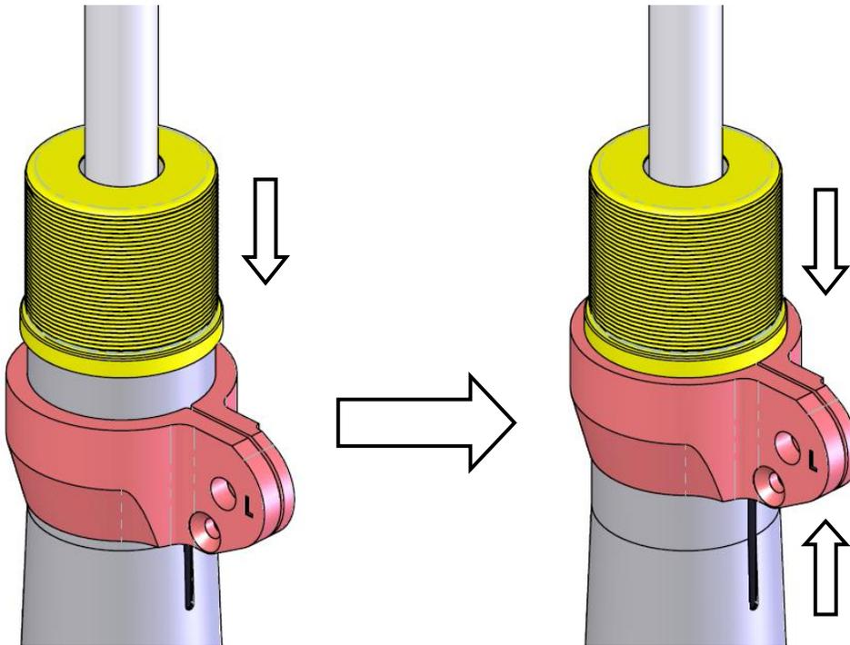
10. See figure above. While pushing down on the threaded sleeve, slide endlink mount straight upward until it just contacts the sleeve, and no further. This is the proper height for the endlink mount. Verify that the gap in the endlink mount is still aligned with your mark.
