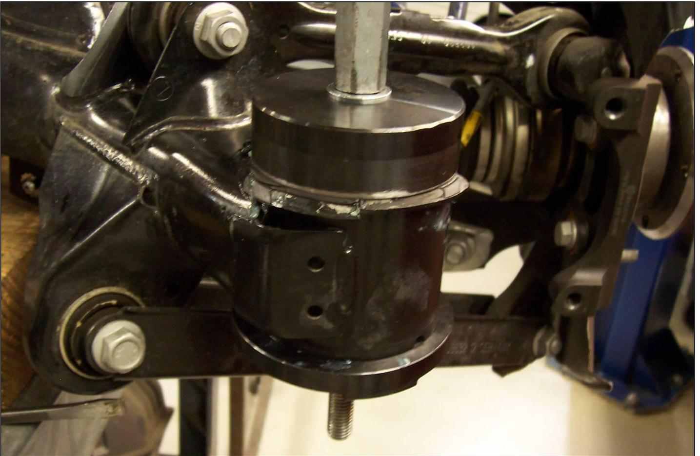
4. When you have all four of the new subframe mounts installed you can reinstall the subframe Assy in reverse order of removal.
