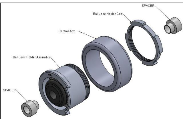
5. Install the Dinan retaining cap onto the arm. Put a small amount of Loctite on the internal threads of the cap and torque to 110 foot-pounds to secure the retaining cap. A special Dinan cap tool is included in every kit. This tool is used with a 1/2" torque drive. Set torque wrench to 110 foot-pounds and do not concern yourself with a conversion factor. See figure below.
