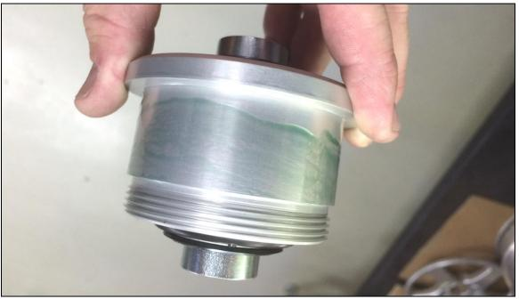
4. See figure below. Slide the ball joint assembly into the control arm. Threads shall be inserted first from the side that has a raise of material on the control arm. While inserting use a slight turning motion to further spread the Loctite around. The ball joint assembly should sit flush against the surface of the control arm. If inserted on the wrong side, the ball joint holder cap will not sit flush against the surface.
