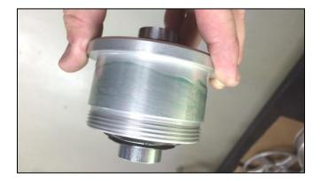
5. See figure below. Slide the carrier into the bore in the arm with a slight turning motion to further spread the Loctite around. It does not matter from which side of the arm you install the carrier, but it is preferred if both sides of the car were the same. The carrier shall sit flush against the surface of the control arm.
