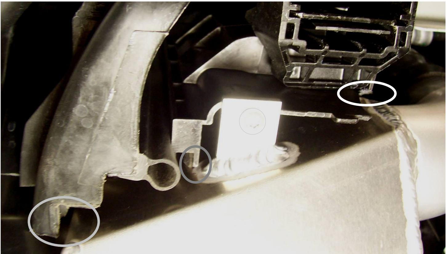
7. The cutting for most of the plastic can be done using a hacksaw and a jig saw. It is easy to cut so don't go overboard as you can always take a little more off later. Minor trimming can be done with a sanding disc or large diameter die grinder bit.
