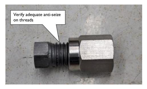
b) Assemble tool with rivet nut as shown.
