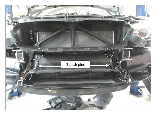
5. Remove the 6 bolts that secure the front brace and remove brace from car. Note that the top two bolts come in from the top. <u>Take care to avoid damaging the fins</u> on the radiator as you slide it past the upper air duct.
