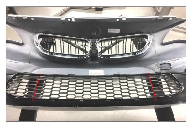
• Measure on the top side of the grill 1/2" on both sides of the center line of the row, as shown in the photo below.
