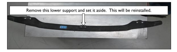
3. Remove the 4 bolts that hold the bumper beam onto the car. Note -- headlight removal is not required for this step.
