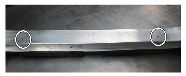
9. Referring to the following steps, install a rivet nut into each hole using the included installation tool. Spare rivet nuts are provided for your use if necessary.
