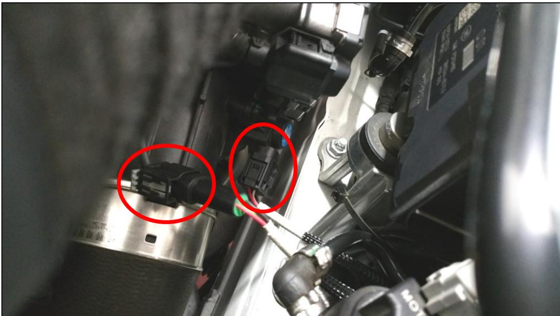
6. The SPORT module is secured using the included zip-ties. Please note -- DO NOT route the zip-tie over the harness at the SPORT module, as this could stress the internal circuit board and damage the module! Only insert a zip-tie thru the slots on the SPORT module as shown below.
