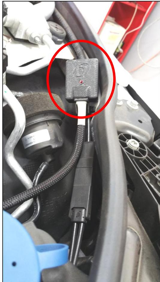
8. Turn on the ignition, but do not start the engine. The LED on the module will illuminate.
