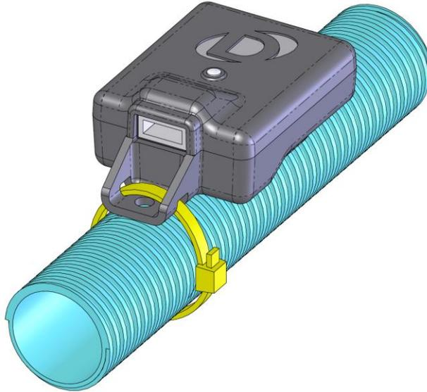
7. Keeping in mind the previous step, mount the module at the location shown. Ensure adequate slack in the wiring harness to allow for engine movement. It is best to orient the module vertically, with the wiring pointing downward.
