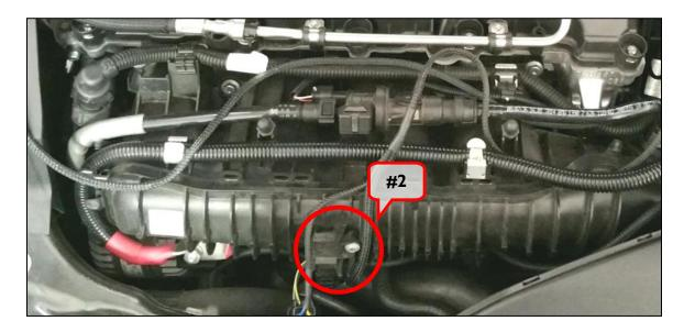
10. Like the previous sensor, install the DINANTronics harness in between the manifold pressure sensor and the factory wiring harness. The connectors are unique, and can only be installed one way. Make sure that the locking tangs on both connections are secure.
