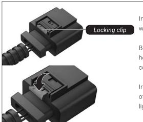
In the first step, the red *locking clip* is pulled out. Press the red *locking clip*, which functions as a lever for loosening the plug and pulling it out.
