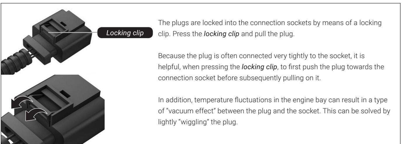
The plugs are locked into the connection sockets by means of a locking clip. Press the *locking clip* and pull the plug.
