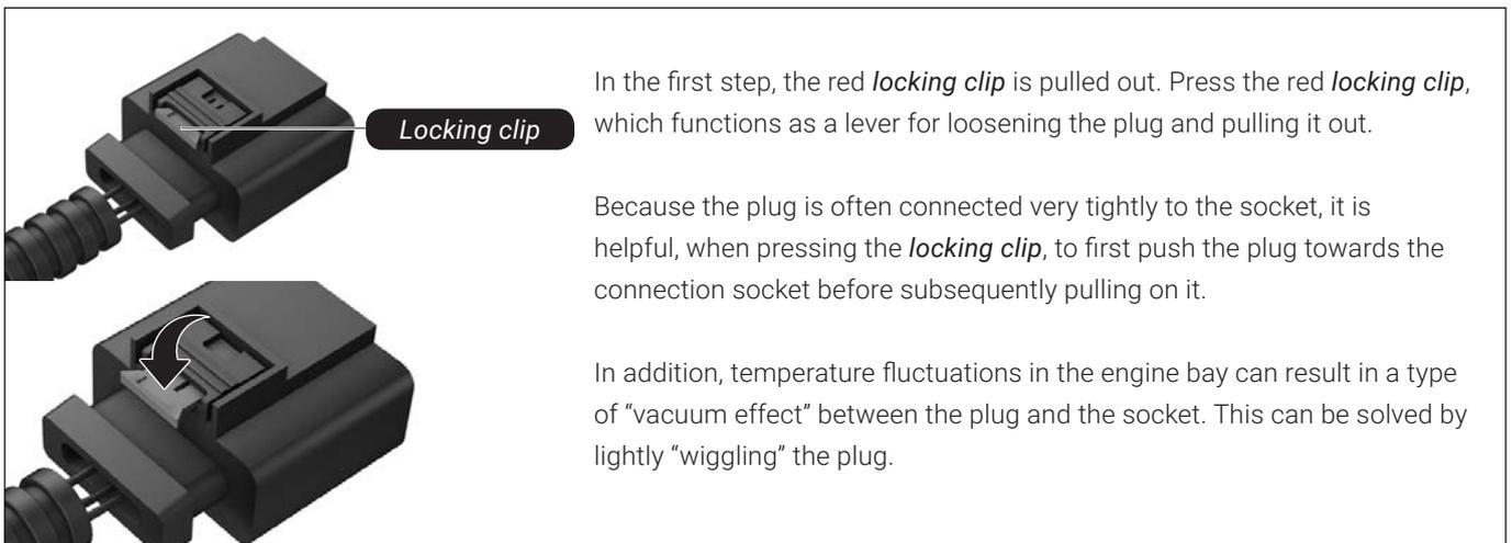
In the first step, the red *locking clip* is pulled out. Press the red *locking clip*, which functions as a lever for loosening the plug and pulling it out.
