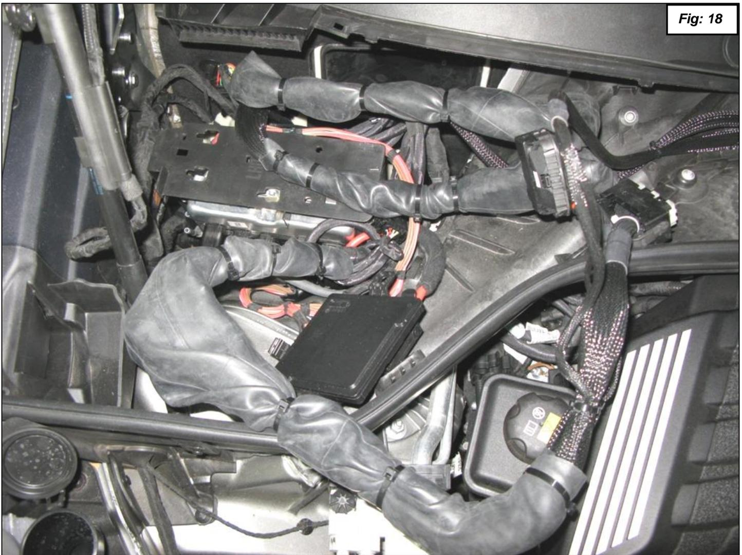
24. Pull the harness interrupt connectors around and connect to the ECU's as shown in the next step making sure you connect them in the correct locations using the previous steps for identification.
