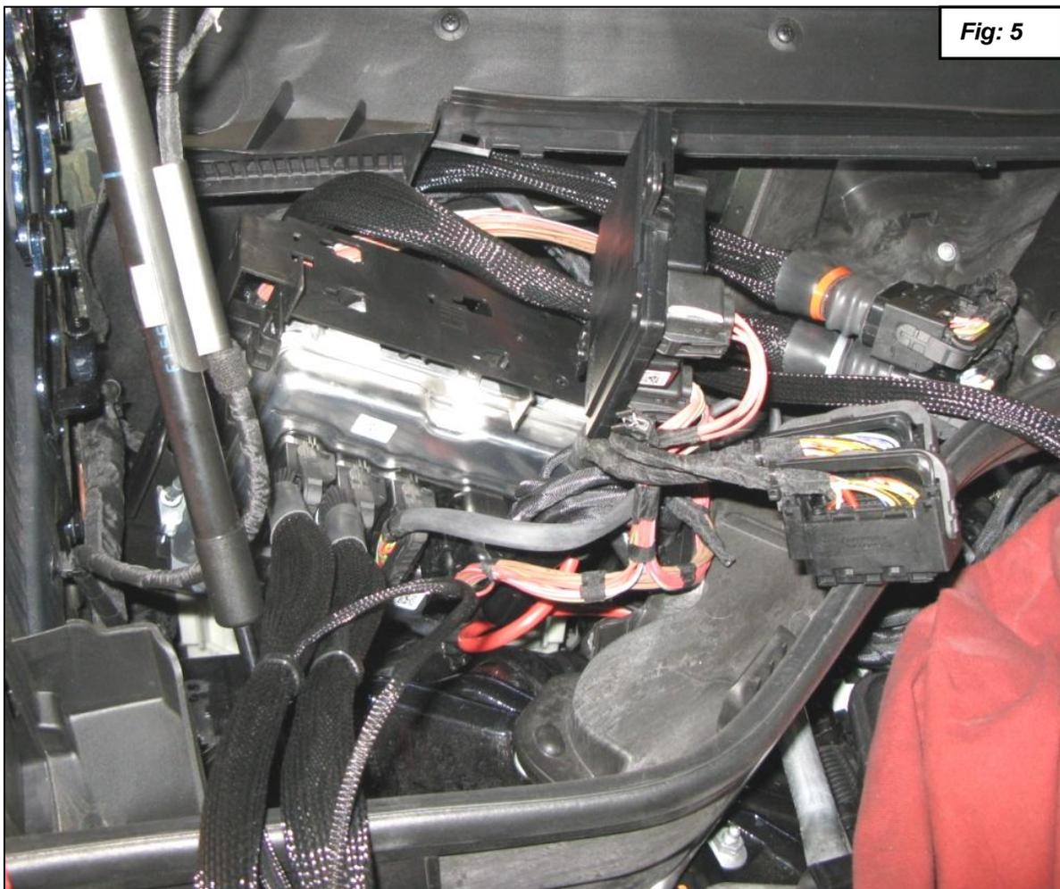
6. There are 2 computers attached to the control unit holder. The control unit for **Bank 1** (1-4) is mounted on the back side towards the fire wall and the connectors are arranged vertically. See figure 6. The front control unit is for **Bank 2** (5-8) and is mounted with the connectors horizontally. See figures 6 and 7.
