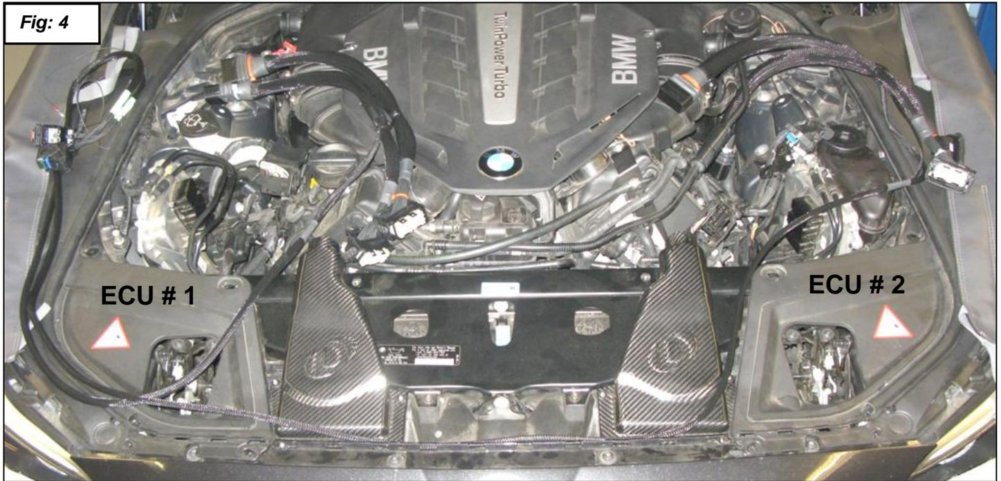
6. The DPT Harness has two pairs of interrupt sections that connect at each stock ECU. They are marked and color coded so you can put them in the right locations. Each connector that connects to the stock ECU's has a numbers on it in addition to the color code.
