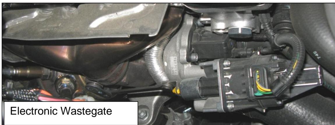
**Wastegate on S55 6-cylinder engines (M3 & M4):**
