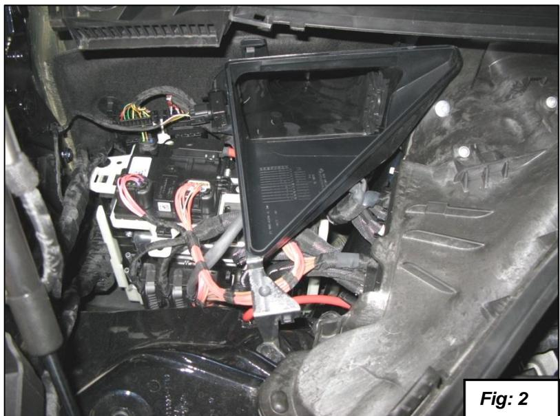
4. Remove the screw holding down the power distribution box. Leave the wires connected to it, detach it from the white plastic holder underneath it, and then pull it over to the side out of the way. Remove the white plastic holder (1) and set it aside until later. See figures 3 and 4.
