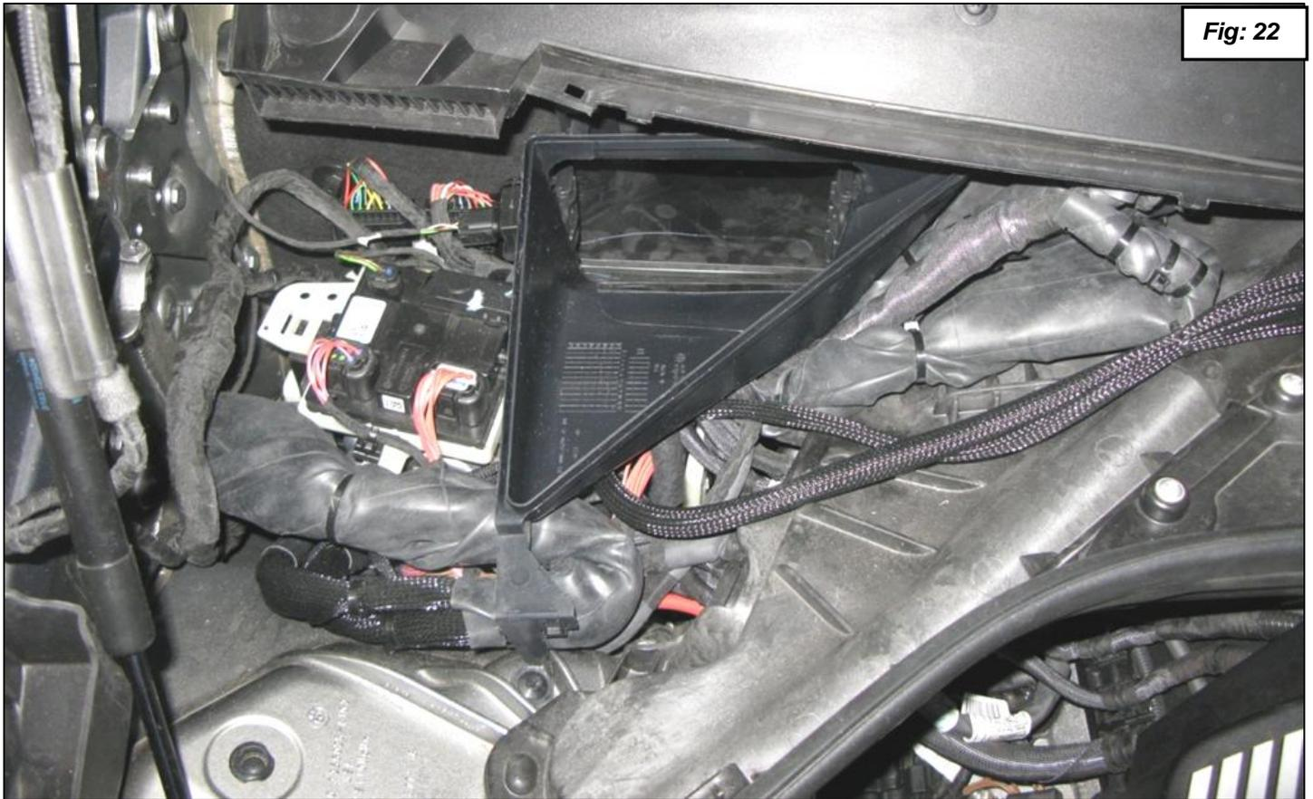
The interconnects for the back ECU (Bank 1) need to be pulled forward as you insert the air duct, snap it back in place then pull the interconnect back around as shown. Keep in mind that the micro filter also needs to go on. It is a tight fit but can be done with a little trial and error. Loop the front interconnects for the front ECU (Bank 2) as shown under the mount for the air duct.
