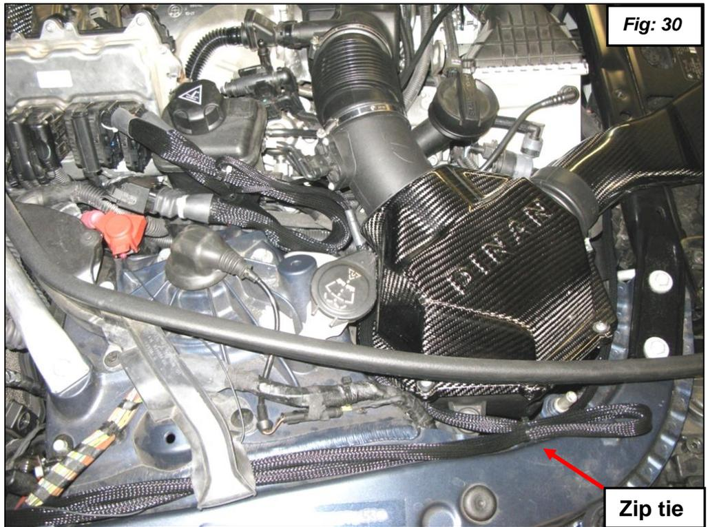
29. On the driver's side after removing the connectors you need to unclip the wire holder and remove the harness as shown in figure 31.
