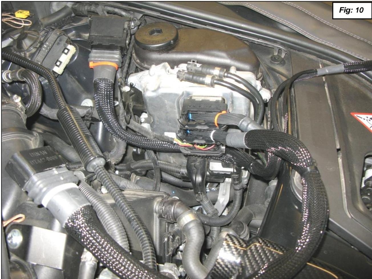
12. Install the Interrupt section that has the White Dot between position (2B) on the ECU and the stock connector that has 4 rows of small connectors, two large connectors and is White in color. See figure 10 and 11.
