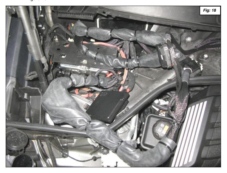
24. Pull the harness interrupt connectors around and connect to the ECU's as shown in the next step making sure you connect them in the correct locations using the previous steps for identification.
