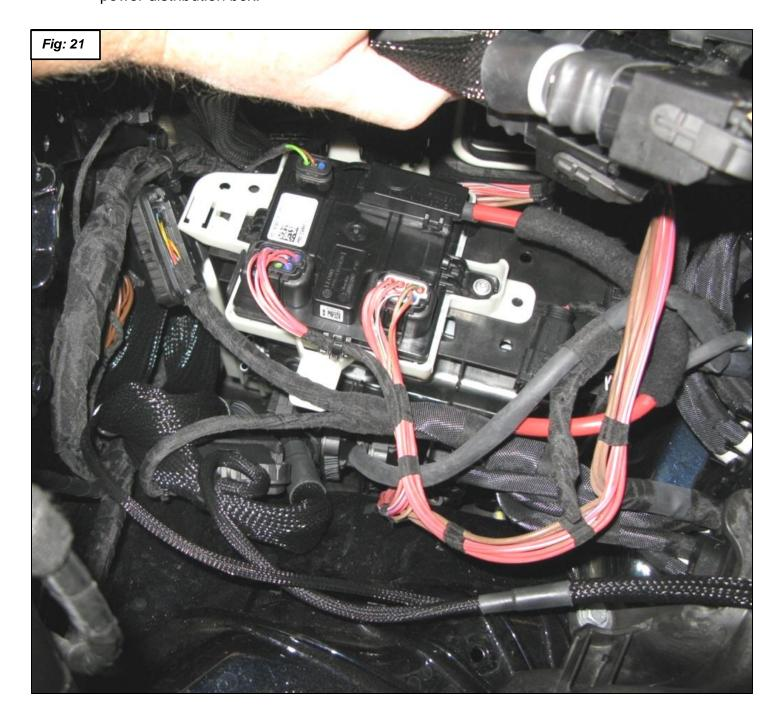
27. Route the wires as shown on both ECU's as shown in figures 22 and 23.
