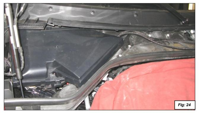
29. Run the wires for the DINANTronics box as shown securing the with the supplied loop clamps using the screws in the engine bay partition. The loop clamps are there to keep the wire out of the wiper arm when it's in motion. See figure 25.
