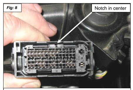
When installing the connectors, use the lube spray and push the connectors into position as far as you can without using the cam lever to pull it in. You will get a better deeper connection; the lever should be loose and not be pushing against its lock.
