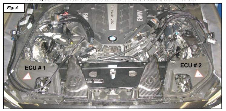
6. The DPT Harness has two pairs of interrupt sections that connect at each stock ECU. They are marked and color coded so you can put them in the right locations. Each connector that connects to the stock ECU's has a numbers on it in addition to the color code.
