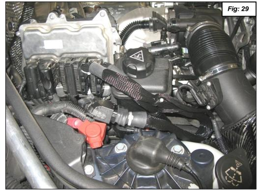
28. Route the two into one splice wires as shown in figure 30 following along the air box. There will be some excess wire, when you get the other side routed around the front of the engine. Zip tie a loop to harness as shown then pull the wire around front to go to the DinanTronics ECU that will mount
