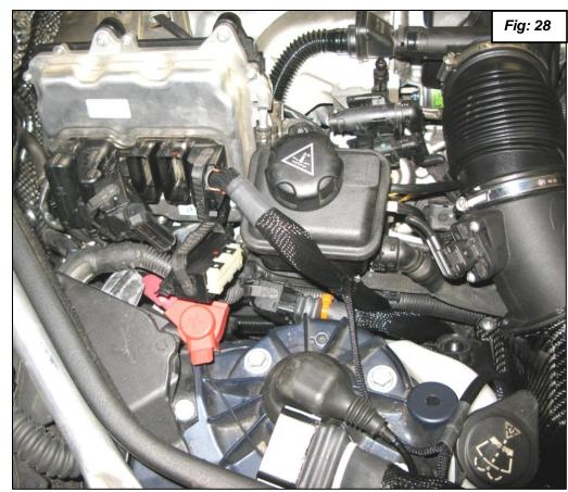
27. Install the White Interconnect between 2B and route as shown in figure 29. Install the last large connector that is the three row plug. It has no interrupt and goes back on as stock in position (1B).
