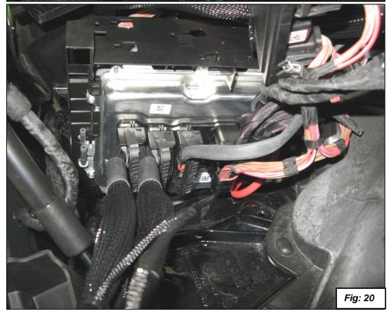
26. Slide the control unit holder down into place while holding up the rear interconnects from Bank 1. The Bank 1 interconnects need to be routed under where the vent duct for interior goes and with the connection to the stock engine harnesses placed up high on the cowl. See figures21, 22 and 23. Reattach the power distribution box.
