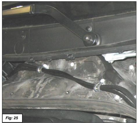
30. Install the DINANTronics box bracket using the wiper motor screw and the screw in the engine bay partition. See figure 26.
