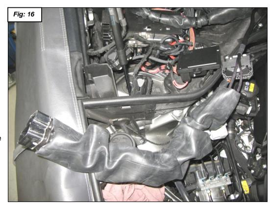
22. Attach all the interconnect connectors together. Pull the rubber as far onto the engine harness as you can. See figures 16, 17 and 18.
