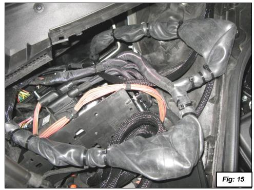
21. On the Front Bank 2 interconnect connectors; slide the large single rubber sleeve over both of the harness interrupt sections as shown in figure 18. Check for sharp corners as before and trim round if needed.
