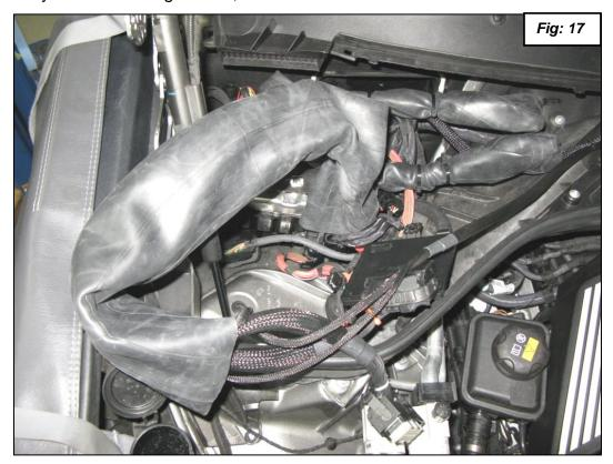
23. Zip tie the rubber sleeve in 3 or 4 spots as needed on each end as shown in figure 20.
