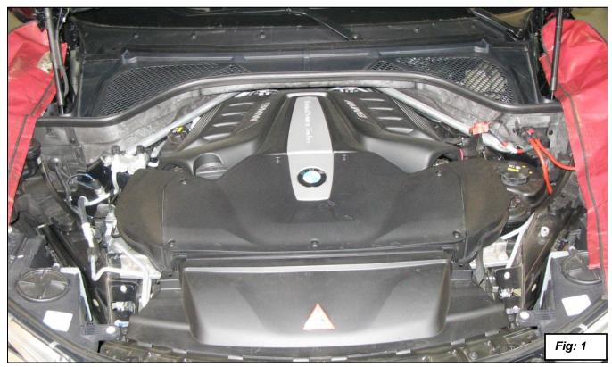
3. Remove the micro filter and the air duct under that. The air duct is held in place in the front with an expanding rivet and two latches inside of the duct. See figure 2
