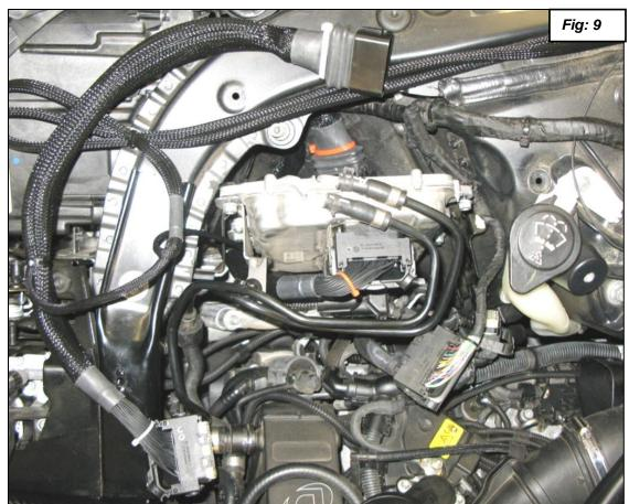
11. The drivers Orange Interconnect wire goes between the three row plug (1B) and the lower connectors as shown in figure 10. Follow the next steps to install the (2B) and (1B) connectors.
