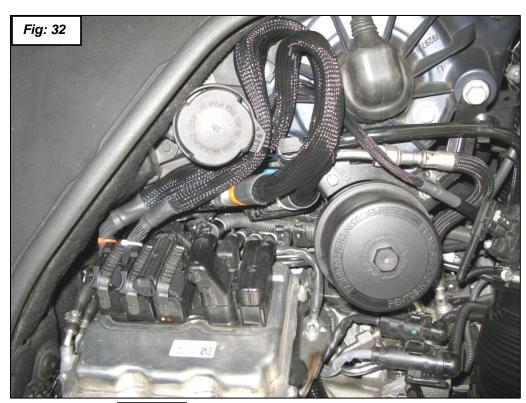
31. Route the wires that go to the DinanTronics ECU around the air boxes to with the excess wire looped and zip tied as show in figures 29 and 32. Zip tie the harness as needed see figures 33 and 34.
