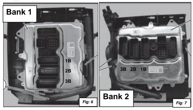
7. Disconnect the first three large connectors on each of the engine control units. See figures 6, 7 and 8. You have to start with the middle large connector (1B) and work your way over to connector (3B). You will be connecting the DPT wire harness connectors between the stock ECU and the stock ECU connectors.
