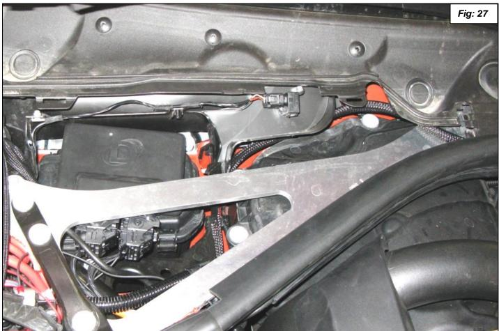
27. If your harness has a external ground wire along with the power wire you need to route it as shown if figure 23. Zip tie it to the stock harness.
