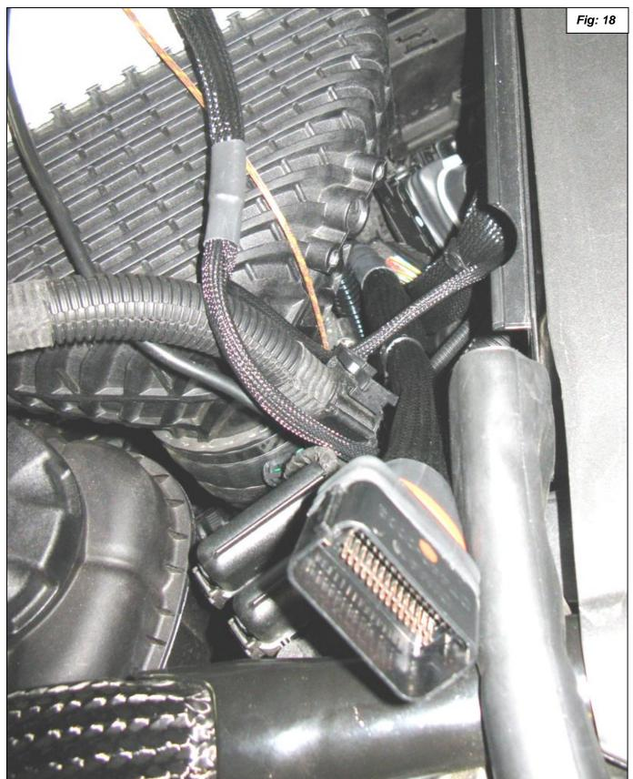
Connect the White Dot Dinan interrupt connector to the stock 2B Wire Harness Connector (Fig: 16) as shown in figure 18.
