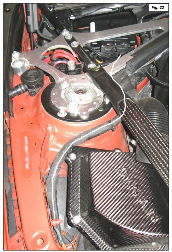
28. Reinstall the cowl cover over the DPT ECU as shown in figure 28. Note: 335i shown for photo clarity.
