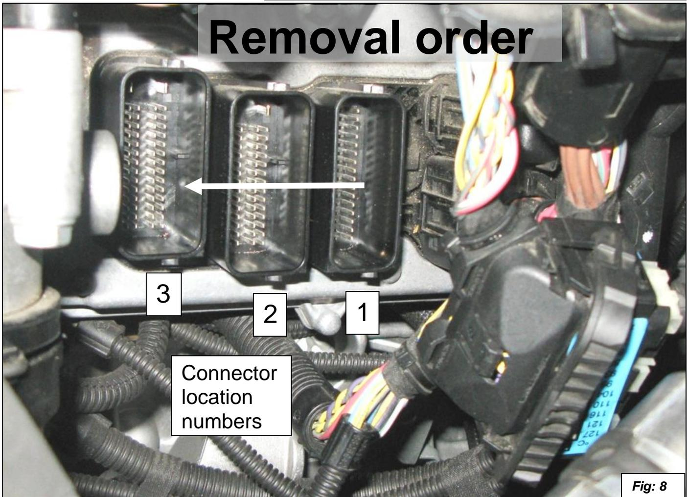
8. Pull the connector number 1 out of the way for now and move the pressure sensor to make room for you to install the Dinan Connectors to the ECU. See figures 9 and 10.
