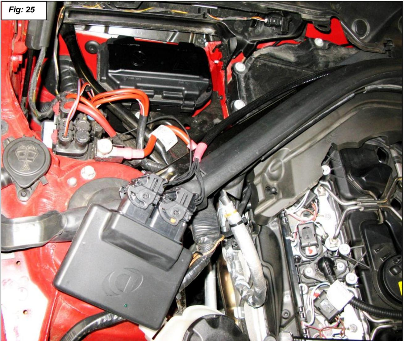
26. Clean the Lid of the Power Distribution Box so the Velcro double stick tape will adhere. Peel the cover off the Velcro and adhere the DPT ECU to the Lid. See figures 25, 26 and 27. Connect the power wire to the positive battery lug.
