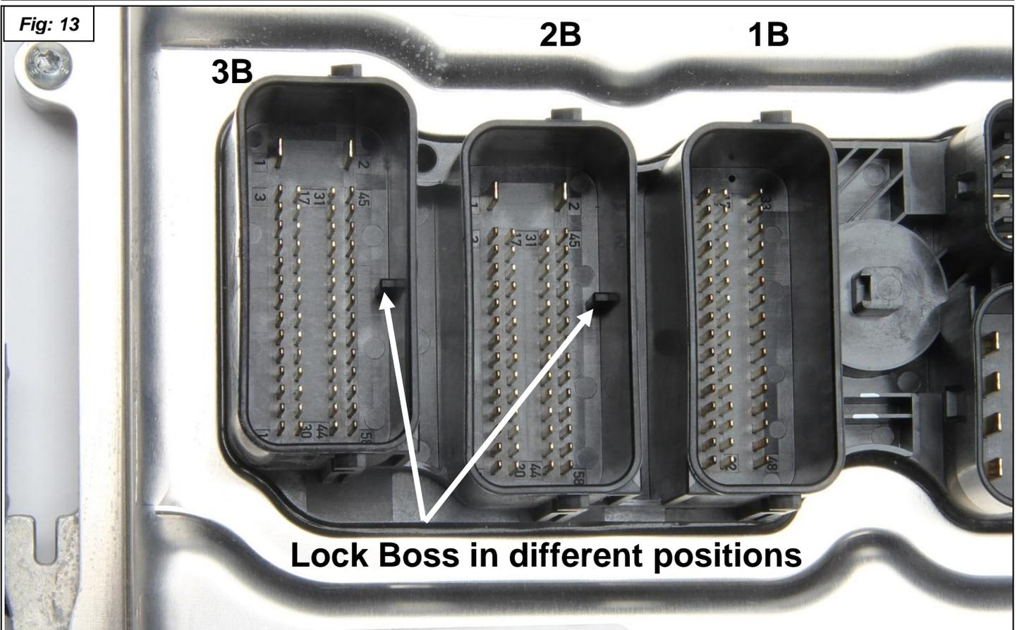
12. The Orange Dot/Zip-Tie Interrupt section gets installed first. It goes between position (3B) on the ECU and the stock connector that has 4 rows of small connectors, two large connectors and is black in color. See figure 14.
