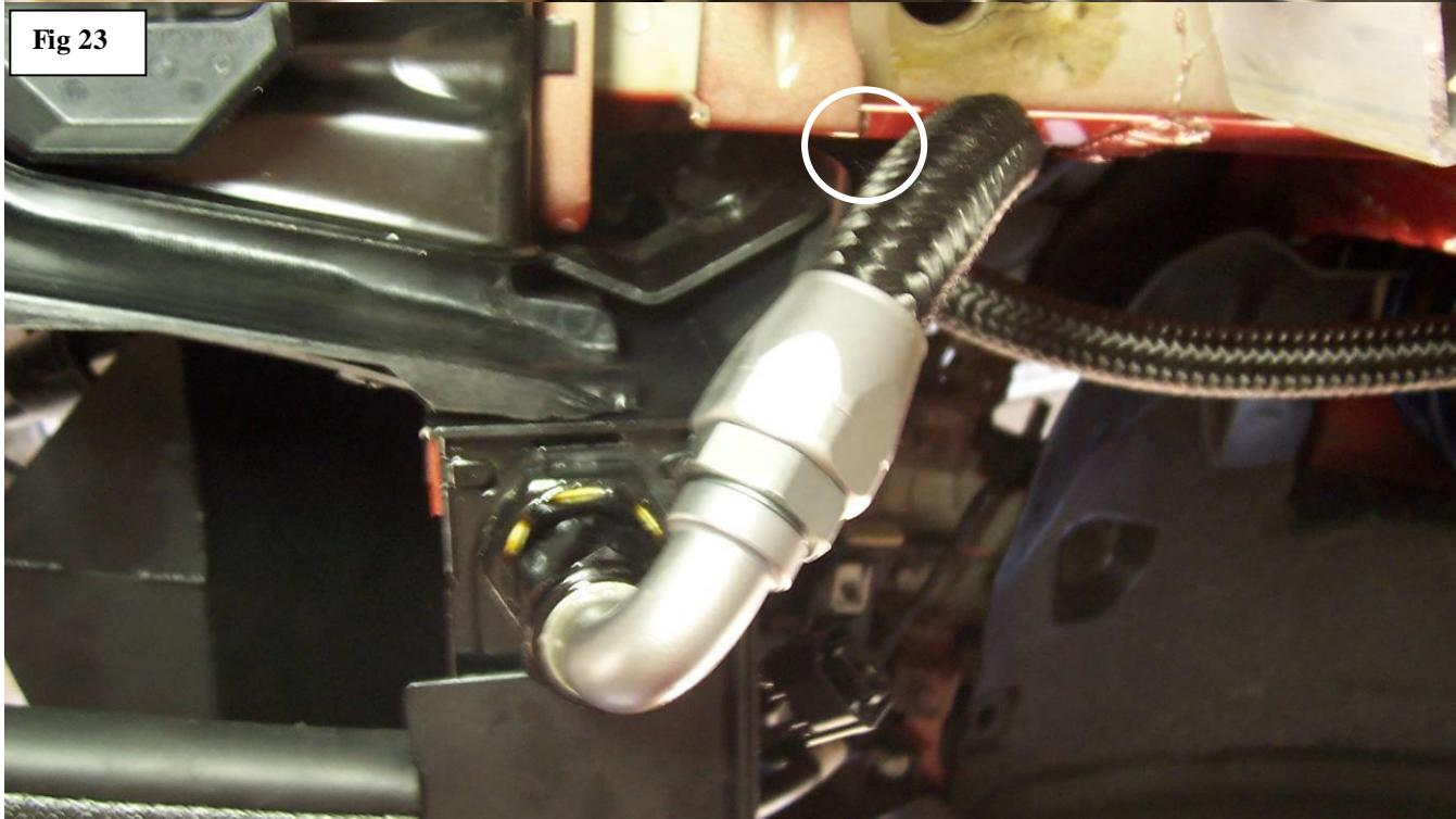
43. You can now mount the modified brake duct. Use the original screw but be careful to not overtighten this screw as you will probably be removing and reinstalling it a few times until you get it right. See the **Figs 22, 23 & 24**.
