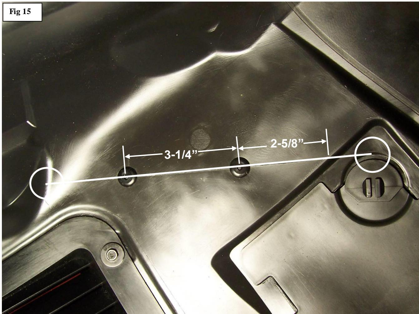
27. Mount the RDC receiver on the front side of the wheelwell liner using the two original rivets with the **connector pointing down**.
