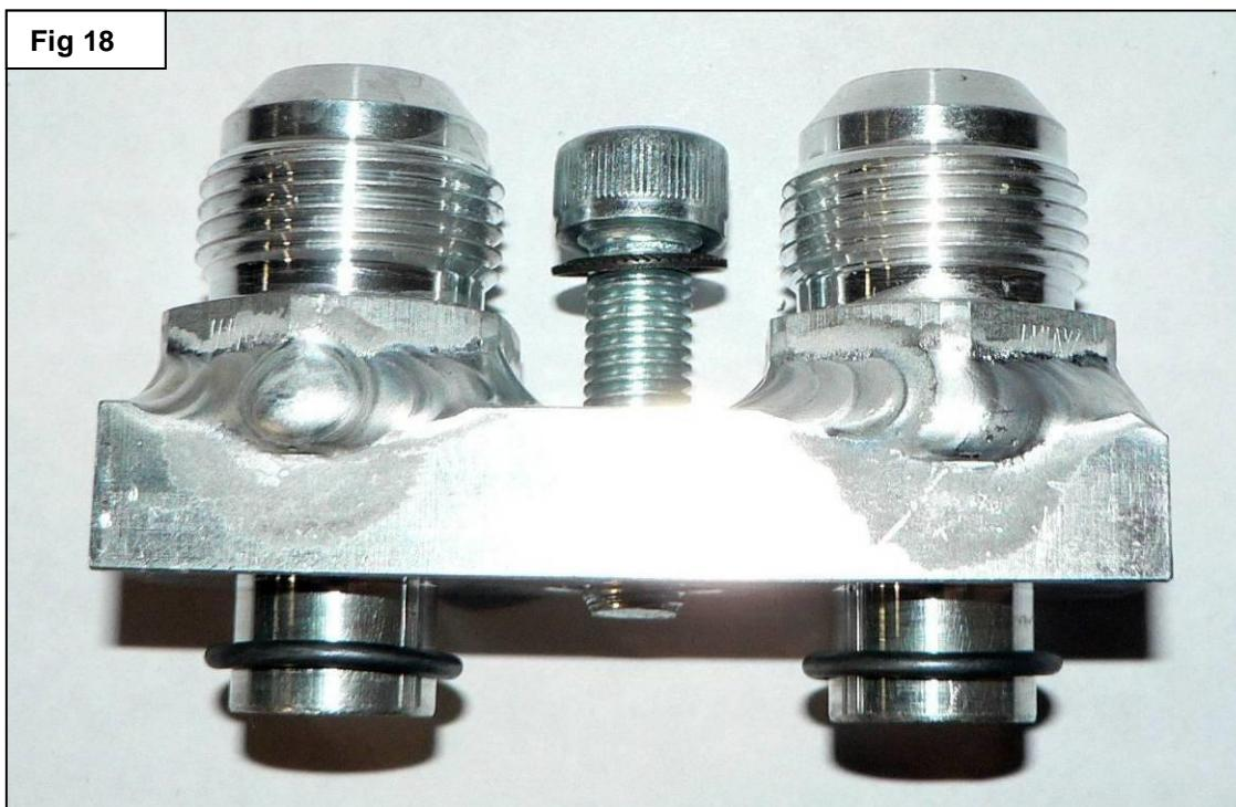
39. Install the Oil Line Mount onto the oil filter thermostat housing. Make sure the O-Rings don't get pinched as you install the block. Hold the Mount up against the thermostat housing firmly as you tighten the screw. Torque the bolt to 20Nm (15ft-lbs.).
