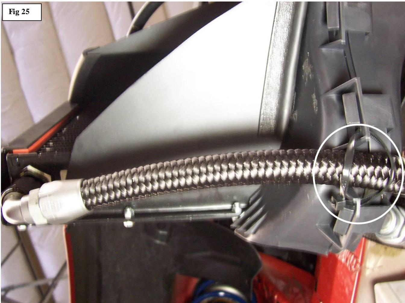
47. After the Oil Hoses are properly routed, use the **Dual Loop Clamp** to secure the Hoses to the upper mounting stud for the Oil Cooler as shown in **Fig 22**. Use the **M8 Locking Flange Nut** to secure the clamp.
