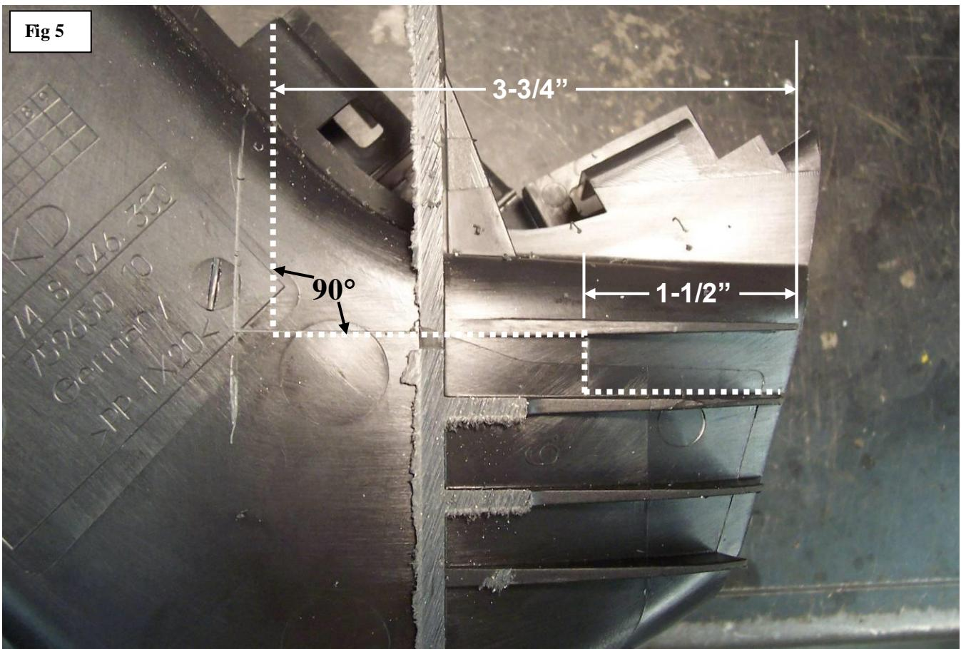
11. Now you can mark the outer side of the right side brake duct. Make the horizontal lines about  $1/16$ " above the "ribs". Note that this duct is already trimmed in the photo.
