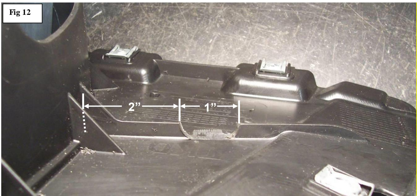
24. Use the photo below to help you measure and mark the small cutout that will allow the wheel well liner to fit around the Oil Cooler.
