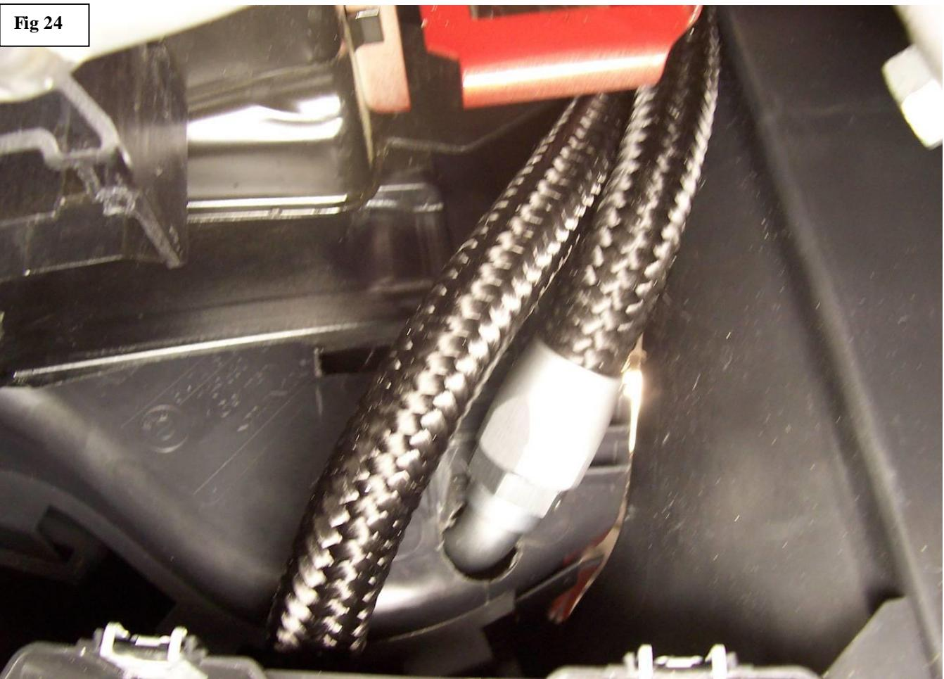
44. When you are satisfied with the fit and routing of the Inner Hose go ahead and **tighten the hose ends**. Note the Hose routing in the previous photos. **Be sure to use a wrench to hold the compression fitting on the Oil Cooler while you tighten the hose end.** Leave a 5/8" to 3/4" gap between the Cooler Hose and the vertical rib on the radiator fan frame.
