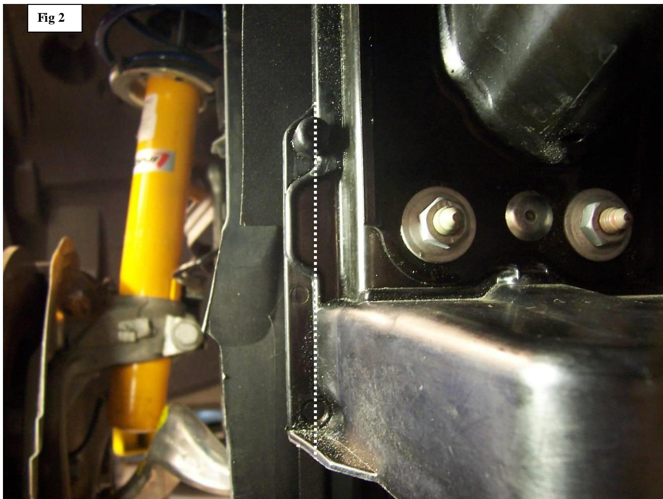
7. Smooth and deburr the cut area where you removed the above edge section. Apply some black touchup paint to any bare metal surface you may have exposed.
