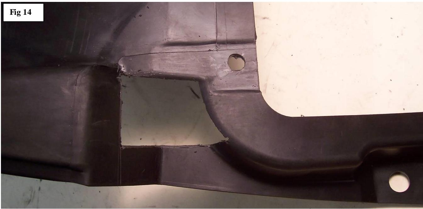
26. You can now relocate the RDC receiver to a higher location on the wheel well liner. Use the photo below to mark a straight line between two points (see circles) then mark and drill two 17/64" holes for mounting the RDC receiver. To prevent the 17/64" drill bit from "wandering" always use a very small bit to drill a pilot hole first. Start the left side of this line roughly at the middle of the curve in the plastic. Note: the receiver is already mounted in place in the photo.
