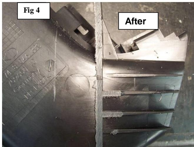
10. Use a small square, a ruler and a sharp scribe to mark the section to be cut on the inner side of the brake duct. Save the silver "captive screw nut" from the piece you cut off. See photo below and next page as well before cutting anything.
