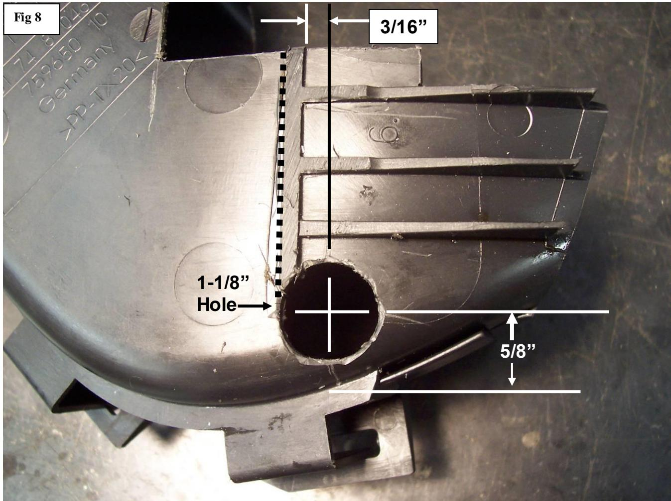
16. Use a die-grinder and a narrow bit to cut a groove in the top of the brake duct as shown below. Make the groove at least  $\frac{3}{4}$ " long.
