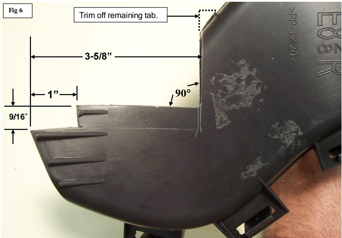
12. Do your best to cut out the section of brake duct that is not needed. You can use a hacksaw to cut the top cut across the duct upper side. Do not cut too much at first - you can easily trim or sand more later.
