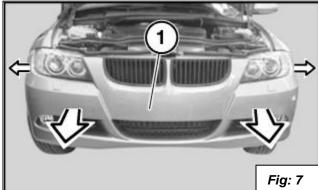
11. Remove bumper trim (1) with the aid of a second person by pulling out at top slightly and forward. See figure 7.
