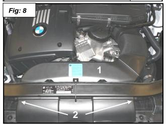
12. Remove the air duct (1) that goes from the top of the radiator to the air box by removing the screws (2). See figure 10.
