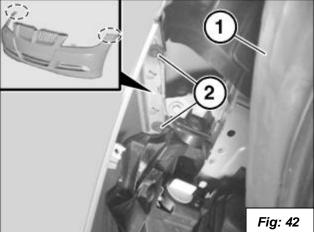
50. Fit the inner fender into position and mark as shown in figure 43 so you can enlarge the opening for the oil cooler vent.
