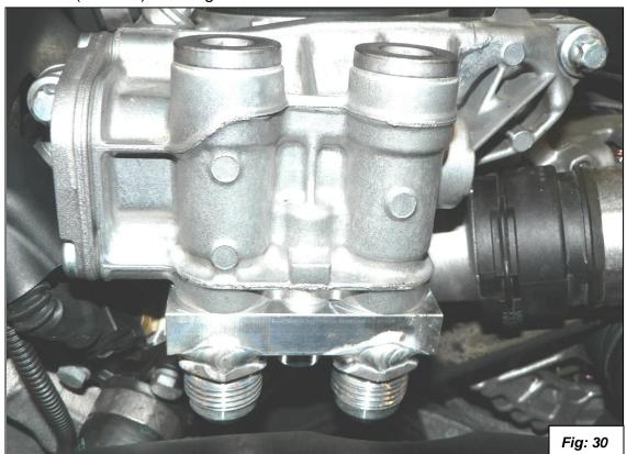
37. Loosely install the oil line with the 90° fittings on each end. One end has a swivel and one end doesn't. Install the end without the swivel onto the topside of the oil cooler. Do not tighten yet. See figure 31.
