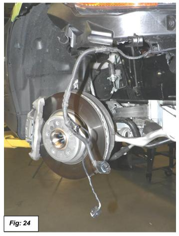
33. Remove the tape and plastic tube that covers the wires as shown in figure 25.
