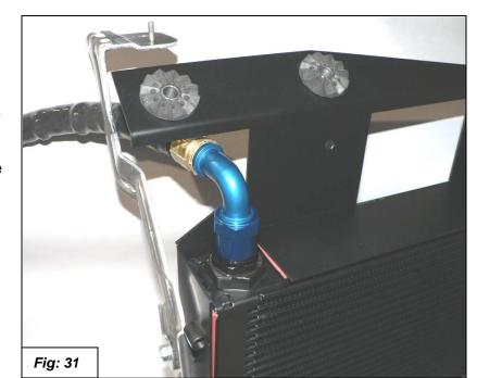
38. Feed the oil line in between the headlight and the bracket as shown in figure 32. Attach the oil cooler assembly to the mounts as shown with the two stock 8mm nuts and the 6mm bolt. Torque nuts to 20Nm (15ft-lbs.) and bolt to 8Nm (6ft-lbs.). See figure 32.
