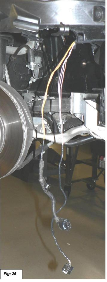
34. Reroute the wire for the transmitter as shown in figures 26, 27 and 28.
