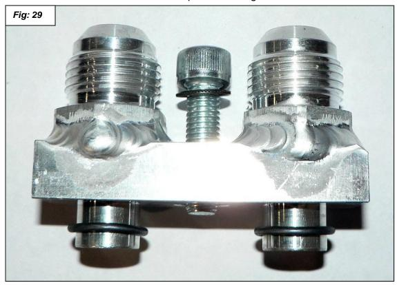
36. Install the oil line adapter block onto the oil filter thermostat housing. Make sure the O-Rings doesn't get pinched as you install the block. Torque the bolt to 20Nm (15ft-lbs.). See figure 30.
