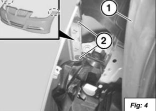
8. Remove the doors for the headlight cleaning system if your car is equipped with them. Pull out spray nozzle (1) by cover (2). Hold spray nozzle and carefully unclip cover sideways and remove. Important! Do not let go of Spray Nozzle when removing Cover! Grip spray nozzle firmly and slowly slide back into bumper after removing cover. Letting it slam back into bumper will damage it! See figure 5
