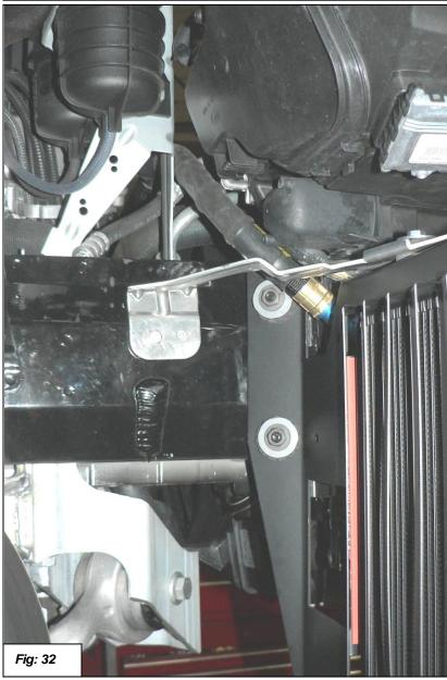
39. Install the 90° swivel end of oil line onto the adapter as shown in figure 33.
