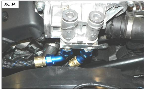
41. Check line for best routing and tighten fittings with 2 wrenches, one on hose fitting and the other on fitting attached to oil cooler or adapter block.
