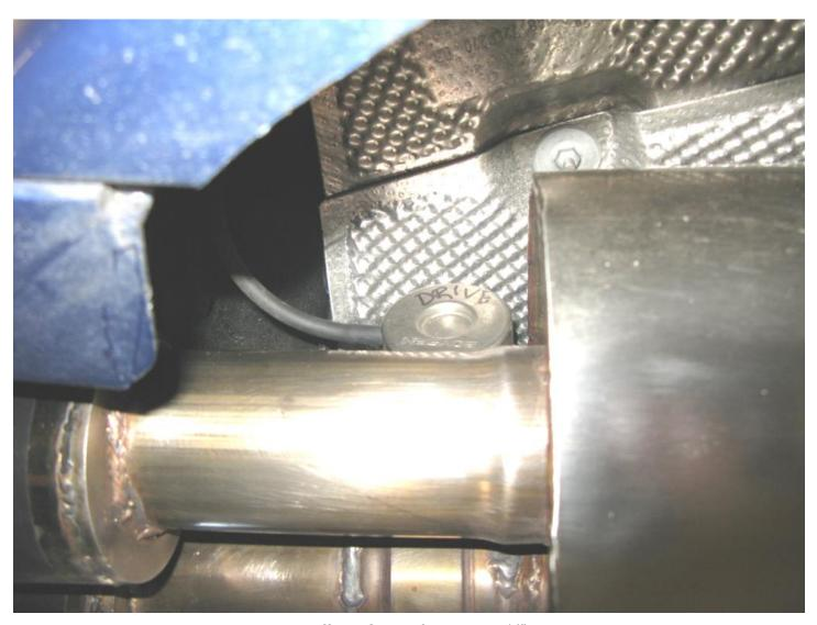
12. Visually inspect the muffler. Check for at least ½" clearance in all areas. You can bend the heat shields slightly if needed.
