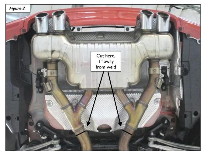
4. With the stock muffler fully secure and supported on a jack or stand, remove the hanger nuts as shown (SAVE THESE NUTS FOR INSTALLATION OF DINAN MUFFLER!). Then remove stock muffler. Be sure exhaust valve actuators are disconnected before finally removing the muffler.
