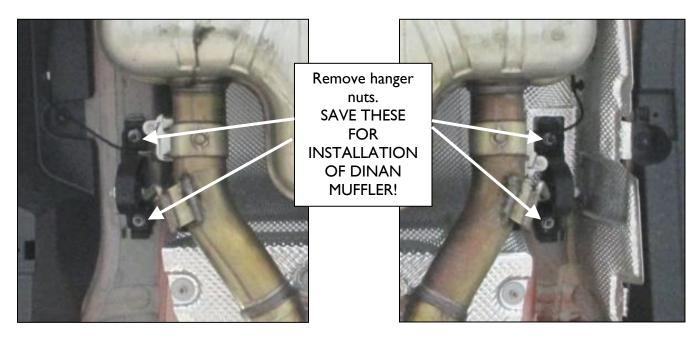
5. Remove stock hangers and valve actuators from stock muffler. SAVE THE HANGERS, HANGER MOUNTING NUTS, ACTUATOR PLATES AND ACTUATORS FOR INSTALLATION OF DINAN MUFFLER!
