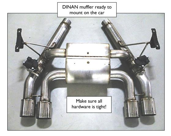
8. Place exhaust clamps provided in the hardware kit onto the ends of the stock exhaust pipes. With DINAN exhaust secured on a jack or stand, put the muffler in place. When mounting the muffler it should be held with the tips up near the bumper and the muffler pushed forward against the ends of the stock pipes.
