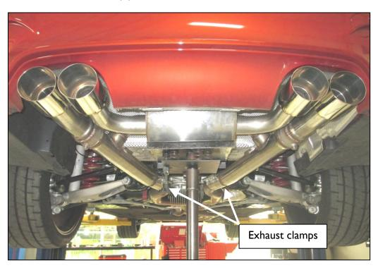
9. Mount both muffler hangers using the stock mounting nuts that were saved from removal of the stock muffler. Torque the nuts to 14 ft-lbs (19 Nm).
