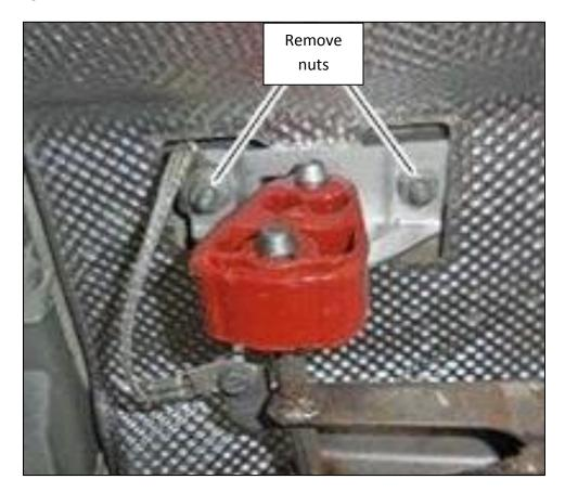
4. Remove (2) hangers, (4) hanger mounting nuts, (2) valve actuators, (2) valve actuator plates,
