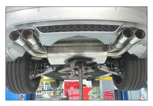
9. Mount both muffler hangers using the (4) mounting nuts that were saved from removal of the stock muffler. Torque the nuts to 14 ft-lbs (19 Nm). Connect ground strap from its stock position to the allen bolt on the DINAN muffler using the nut provided in the hardware kit.
