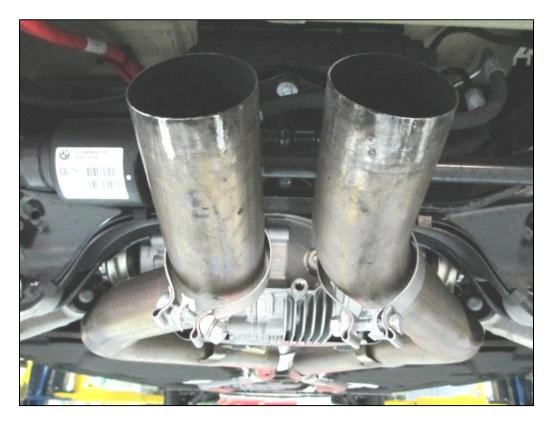
8. With the DINAN muffler secured on a jack or stand, put the muffler into place. When mounting the muffler it should be held with the tips up near the bumper and the muffler pushed forward over the stock exhaust tubes.
