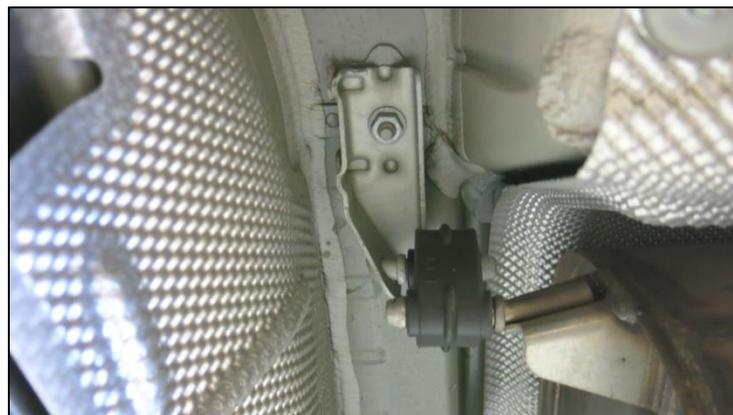
7. Lower muffler out of the car.
