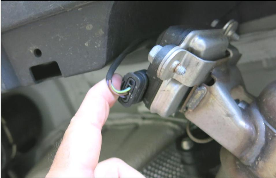
6. Support the stock muffler with a stand and remove the nut on each side of the muffler holding the hanger brackets to the chassis.
