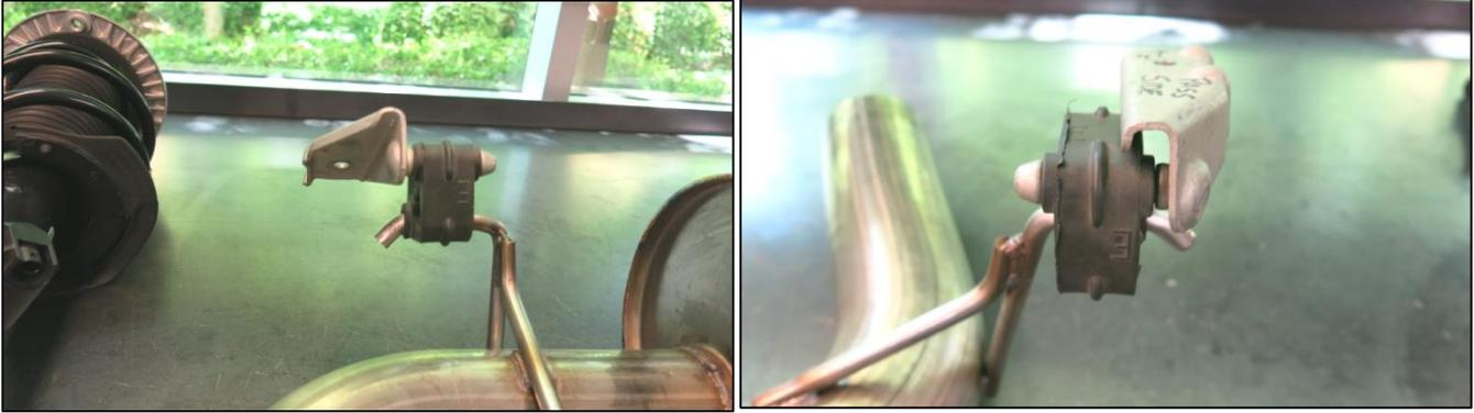
13. Slide the included muffler tube clamp over the exhaust tube. Install muffler with the clamp evenly over the exhaust tube and muffler tube as shown, and gently snug the clamp bolts. Then finish hanging the muffler using the stock left and right hanger nuts.
