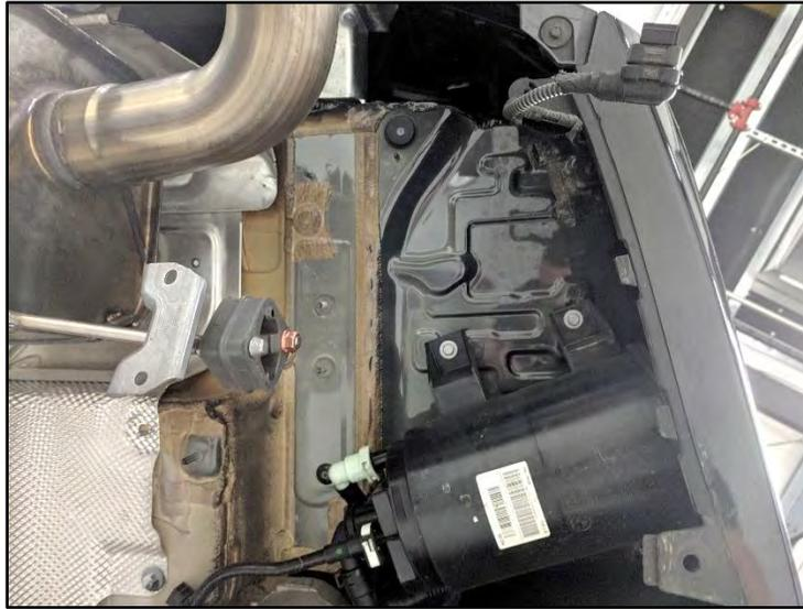
6. Relocate the exhaust valve motor:
