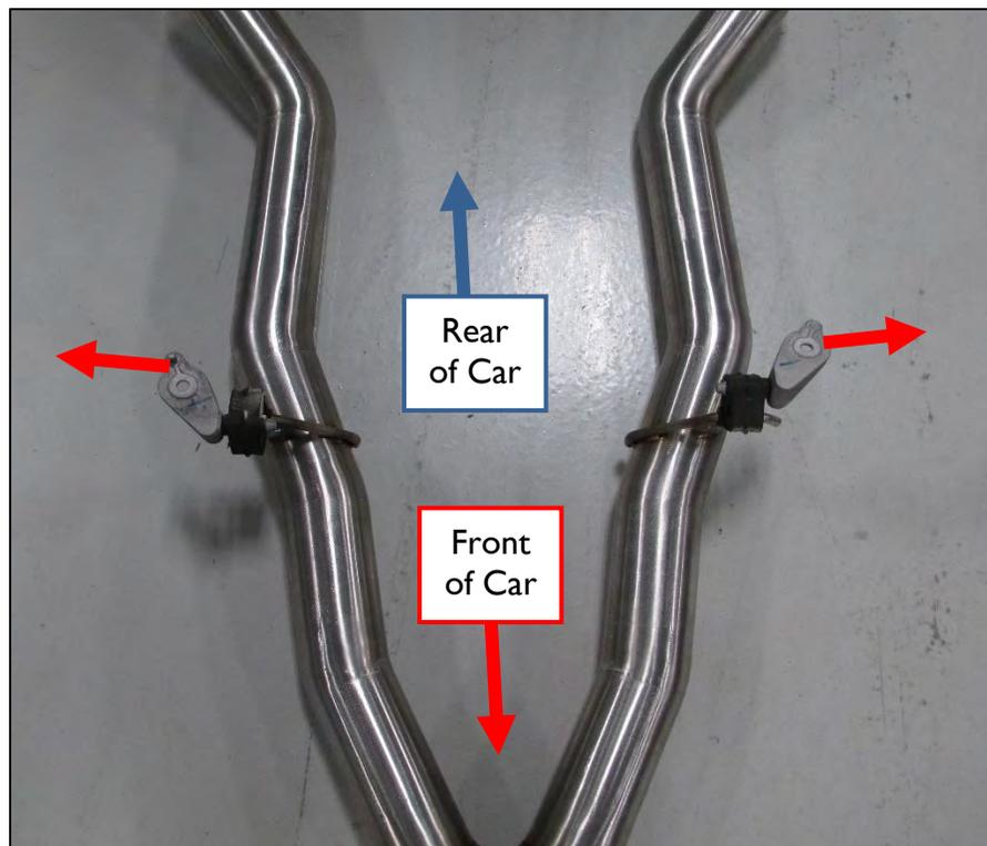
11. Lift the Dinan rear section into vehicle and attach the hangers to the car using the hardware previously removed.
