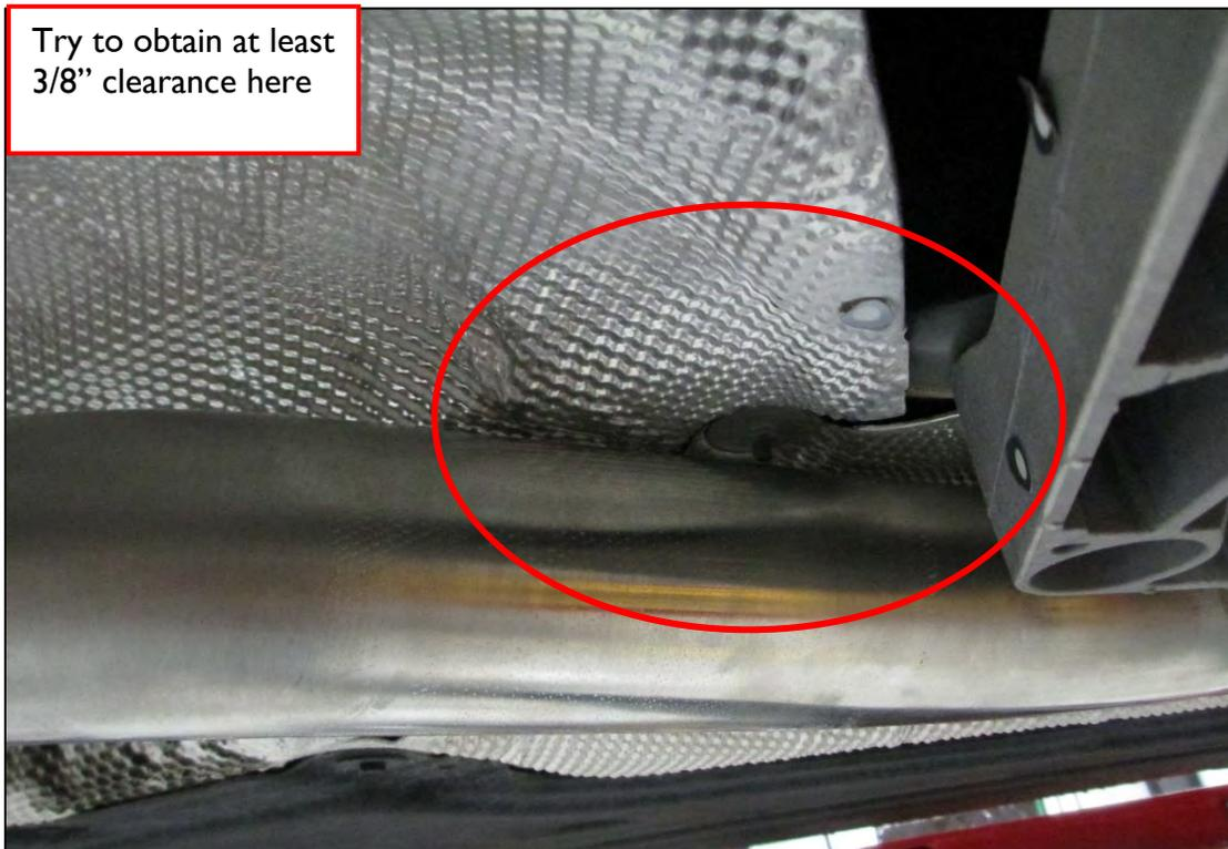
15. When satisfied with the fit, fully tighten all clamps, starting at the front, and working your way to the rear, making any final adjustments as needed.
