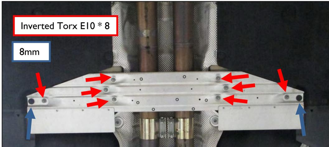
3. Unbolt and remove the stock middle exhaust from the car. Leave the rear muffler in place, attached to the car. Set any hardware aside, as they will be reused.
