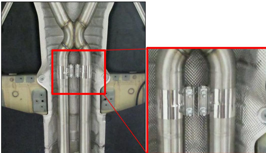
14. The driver's side inlet pipe requires additional attention. There is minimal clearance between the pipe and the underside of the car, near the transmission brace. Adjust the pipe to maximize the clearance in this area, as shown in the following photos.
