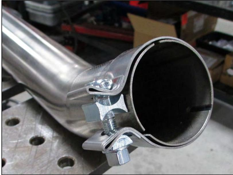
6. Lift inlet pipes into the vehicle, making sure the clamp hardware is on the inside, to avoid contact with the body.
