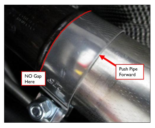
Join the rear sections of the two inlet pipes using the supplied wide clamps, arranging the clamp hardware to avoid contact with the body.
