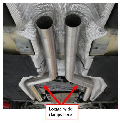
9. Slide the remaining Dinan double clamps onto the inlet pipes, with the hardware towards the middle of the car, as shown below.
