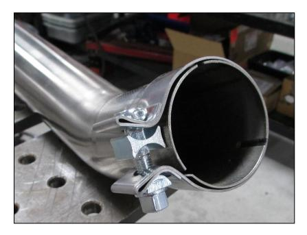
6. Lift inlet pipes into the vehicle, making sure the clamp hardware is on the inside, to avoid contact with the body.
