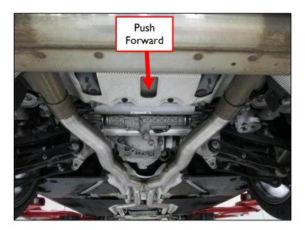
13. For best performance, center the two middle clamps evenly onto the inlet pipes, and the rear section pipes as shown.
