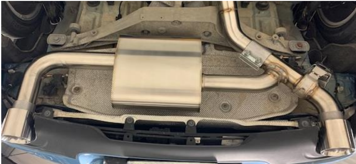
Figure 7: Exhaust Hanger Installation
