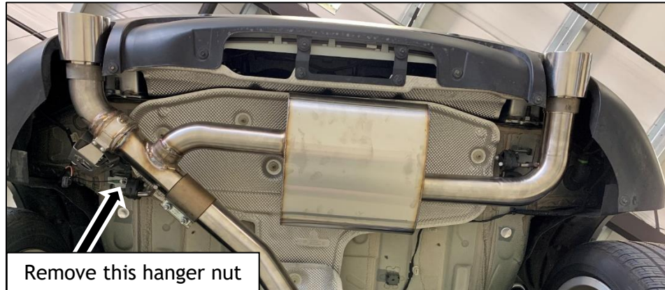
Figure 30: Hanger Ground Location
