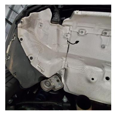
9) The muffler cavity should look like the picture below.
