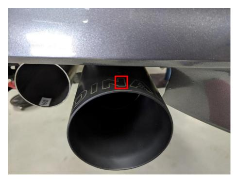
19) The exhaust tips should fit on both sides as pictured below. Torque the exhaust tip clamps to 45 ft-lbs.
