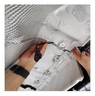
8) Secure the driver's side panel back in place. You may need to adjust this cable length later.
