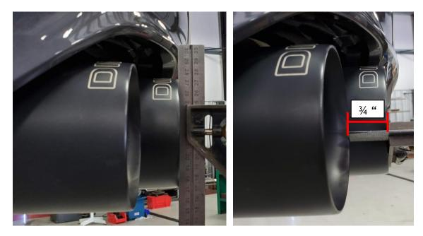
18) After adjusting the tip length and alignment, make sure the second vertical line of the N in the Dinan logo is facing straight up on all 4 tips.
