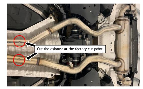
1) Support and cut the stock exhaust at the factory cut point.
