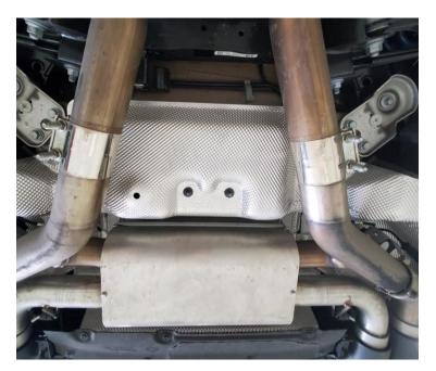
13) Adjust the wiring length on either side to allow the valve motors to plug in. There should be sufficient slack on each side to allow for movement but without rubbing against or contacting anything.
