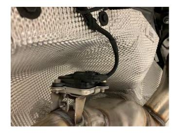
3) Unbolt the exhaust hangers and remove the stock muffler.
