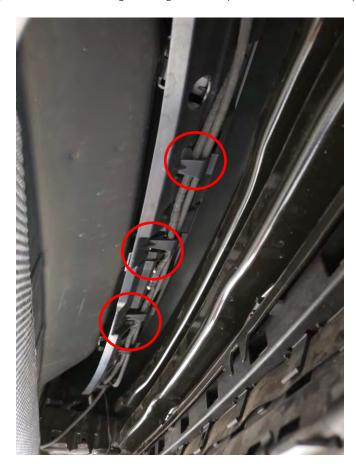
7) Loosen the driver's side panel and route the wiring as pictured below. Leave about 8 inches of wiring length on this side.
