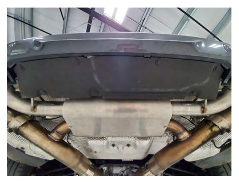
16) Push the muffler up and forward then torque the clamps. If the muffler contacts any part of the car, twist the inlet pipes to adjust. Allow for the pipe clearances as pictured below.
