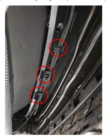
7) Loosen the driver's side panel and route the wiring as pictured below. Leave about 8 inches of wiring length on this side.
