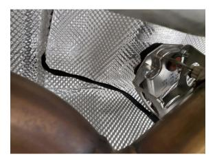
14) Once the wiring is adjusted, cable tie the newly installed exhaust valve cable in three places to the preexisting cable in the rear bumper and trim the excess cable tie.
