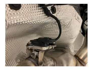
3) Unbolt the exhaust hangers and remove the stock muffler. For G23 & G26 - remove stock braces as needed.
