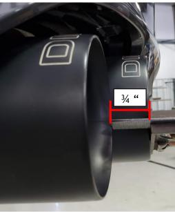
19) After adjusting the tip length and alignment, make sure the second vertical line of the N in the Dinan logo is facing straight up on all 4 tips.
