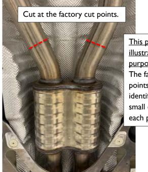
This photo is for illustrative purposes only. The factory cut points are identified with small dimples on each pipe.
