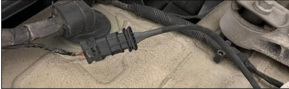
Figure 3: Attaching the Dinan Harness
