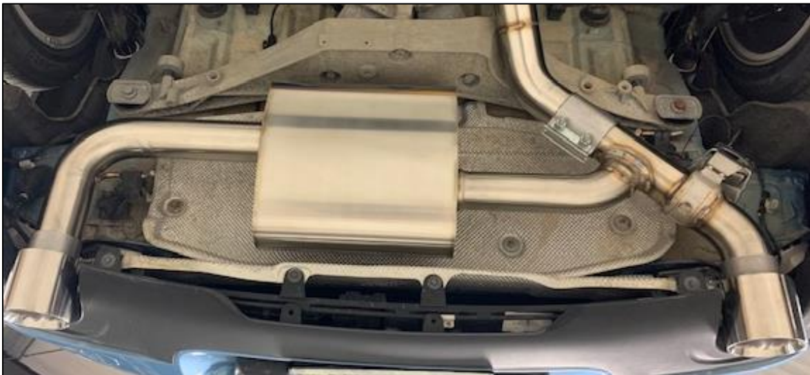
Figure 9: Exhaust Hanger Installation
