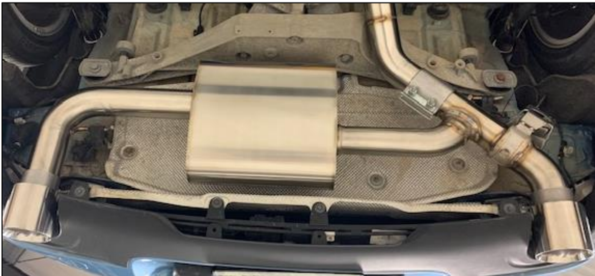
Figure 9: Exhaust Hanger Installation
