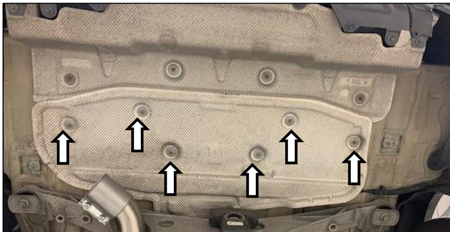
Figure 4: Removing Exhaust Heat Shield
