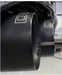
18) After adjusting the tip length and alignment, make sure the second vertical line of the N in the Dinan logo is facing straight up on all 4 tips.
