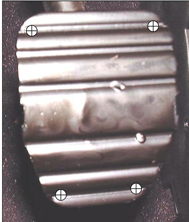
11. Remove the Dinan cover. Centerpunch the marked holes and drill 3/16" holes at the locations you marked. A sharp drill bit is essential for this job.
