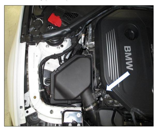
2. Depress the grey tab to release the connector, and detach from the sensor. Move the harness aside.
