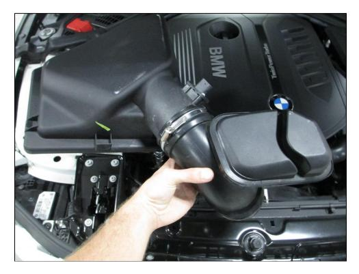
7. WARNING – the turbocharger inlet is now exposed. Items which fall inside can cause severe damage to the turbo! Be sure to place a rag or towel in the inlet to protect the turbo.
