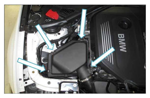
5. Follow the outlet of the airbox, down to the hose clamp near the turbocharger inlet. Loosen this hose clamp. A long extension and universal joint would be very helpful with this step.
