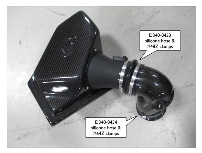
16. Remove the rag from the turbocharger inlet, and install the Dinan intake into the vehicle. Adjust positioning of the intake tube to best clear the radiator bracketry (see below).
