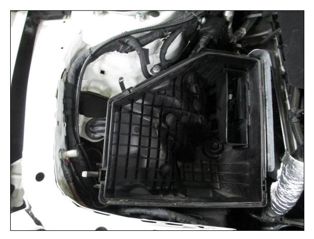
12. Clean out the track around the outside of the lower air box. Insert the adhesive gasket strip into the track after cleaning. Peel off the adhesive backing, install, and trim as needed to fit.
