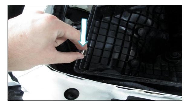
II. Install the Dinan spring clips into the lower airbox. The lower airbox should look like this:
