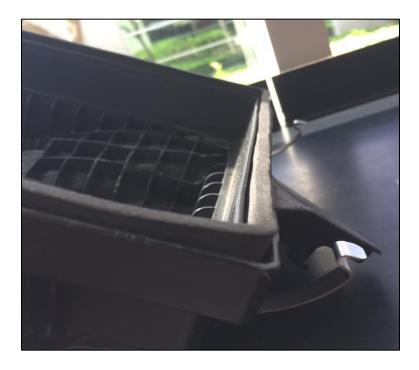
12. Referring to the figure below, attach the Dinan air mass meter to the carbon airbox lid using the 5mm bolts, round & rectangular washers, and nuts as shown. The air mass meter only fits one way.
