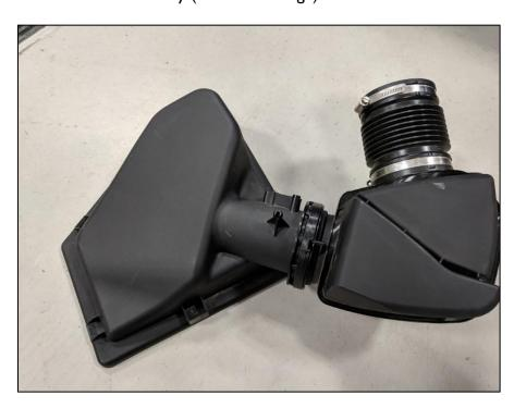
WARNING – The turbocharger inlet is now exposed. Items which fall inside can cause severe damage to the turbo! Be sure to place a rag or towel in the inlet to protect from debris.
