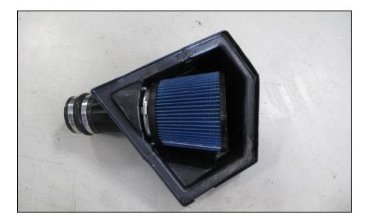
14. Attach the Dinan intake tube and silicone hoses using the included hose clamps as shown below. Leave the hose clamps slightly loose for now, so the intake tube can be adjusted into position later.
