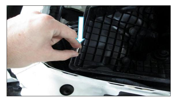
10. Install all the Dinan spring clips into the lower airbox. If needed, remove the lower airbox to install the clips as pictured below. Seat as shown below. Push bottom of clip over lip until snaps into place. Press down to fully seat the spring against the box.
